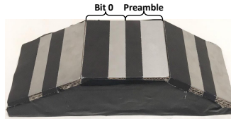
Figure 5.22: The object-ID (preamble + ID value “0”) that is attached to all the three parts of the object.
