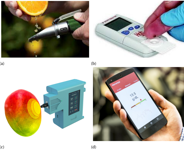
Figure 1.1: The change of sensing paradigm from invasive to non-invasive. The top row displays invasive solutions. (a) Shows a brix evaluation that requires opening the fruit to extract its juice [4]. (b) Shows a test that requires piercing the fingertip to extract blood [5]. The bottom row shows alternative non-invasive solutions. (c) Shows a brix evaluation that relies on mmWave signals and does not require opening the fruit [6]. (d) Shows a hemoglobin concentration test that simply requires placing a fingertip over a smartphone camera [7].
