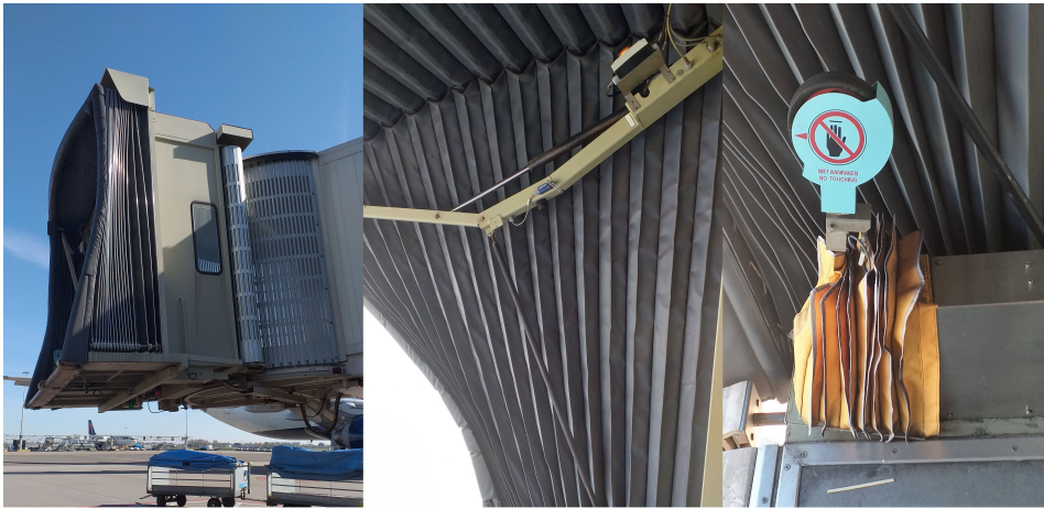
Figure 2.4: The cabin of the PBB seen from the outside, the canopy and the trim arm
