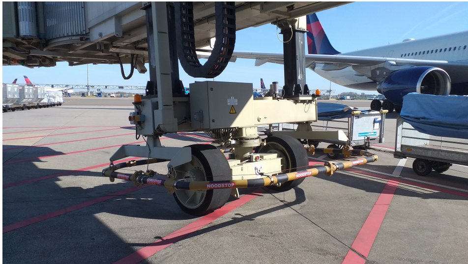
Figure 2.2: The wheel bogies and the elevation system of the PBB
