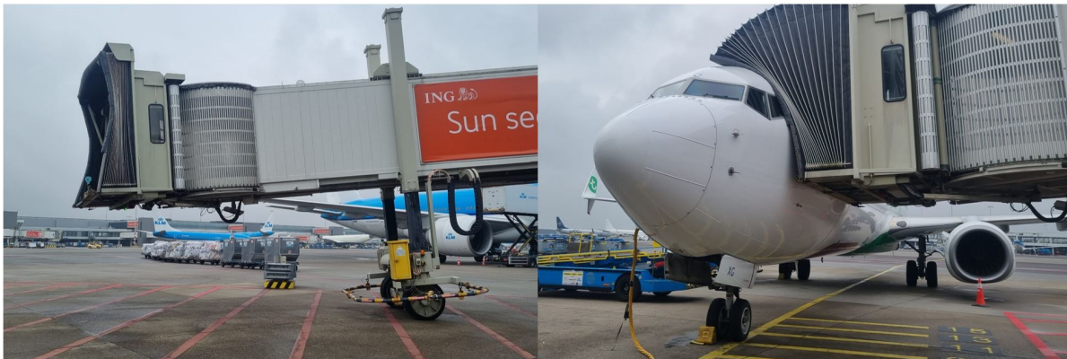
Figure 2.5: The two starting situations of the PBB. On the left is the parking position, and on the right, it is connected to the aircraft.
