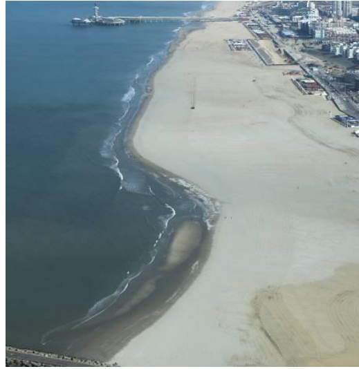
Figure 5: Nourished beach of Scheveningen in 2010. Groynes 42 to 44 are covered by the nourishment, 45 still present. (source: projectbureau Combinatie Delftlandse Kust)
