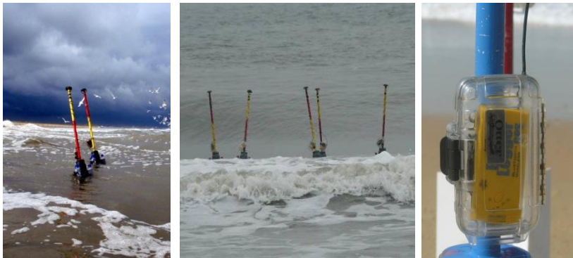
Figures 8, 9 and 10: GPS data loggers attached to PVC buoys. (GPS drifters)
