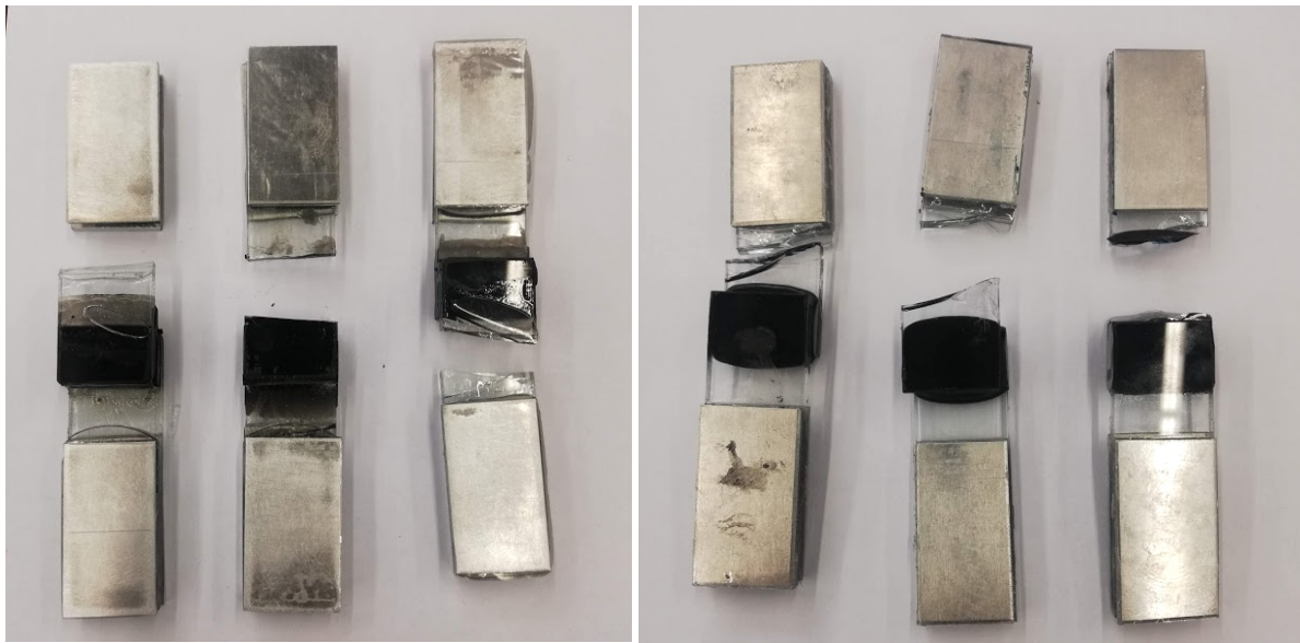
Figure 7.4: Glass failure in UV cycle after 350 hours (a) and TC cycle after 700 hours (b)
