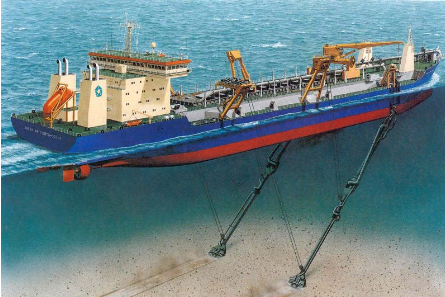
Figure 7.7: Trailing Suction Hopper Dredger (Source: http://www.theartofdredging.com )
