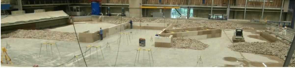
Figure 5.5 - The scale model during construction
