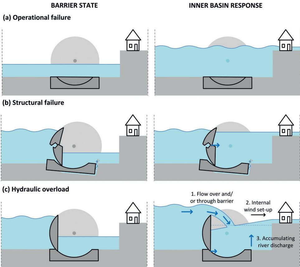
**Figure 2.3:** Principal system failure mechanisms. The left figure presents the barrier (failure) mode, while the right figure shows the corresponding inner basin response, which leads to exceedance of the critical water level.
