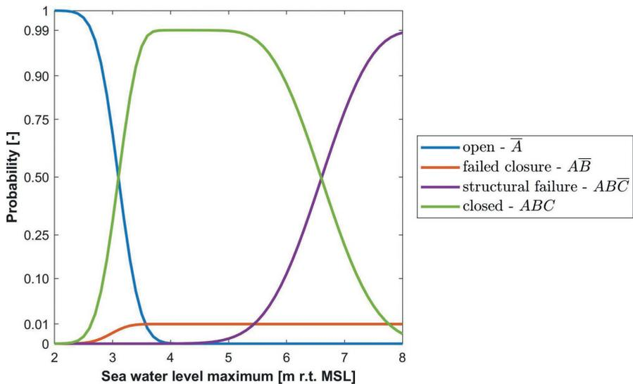
**Figure 2.7:** Example of barrier state probability functions used for the Maeslant barrier case study. Sea level maxima are presented in meters relative to mean sea level [m r.t. MSL]. The vertical axis was scaled using a beta distribution (2,2) to emphasize probabilities near zero and one. The symbols in the legend correspond with the events as indicated in the event tree of Figure 2.6.
