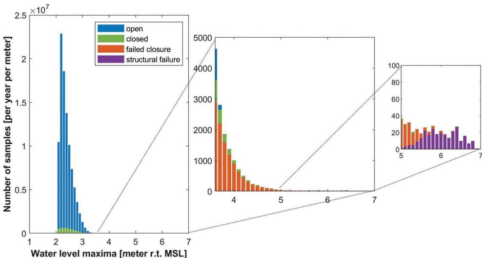
**Figure 2.13:** Histograms with the number of samples from the Monte Carlo Simulation ( $10^8$  samples) that resulted in an inner water level maximum (bins 0.1 meter). The left figure presents all samples and the middle figure presents those which exceeded the critical water level. The right figure zooms in on water levels exceeding MSL+5m.
