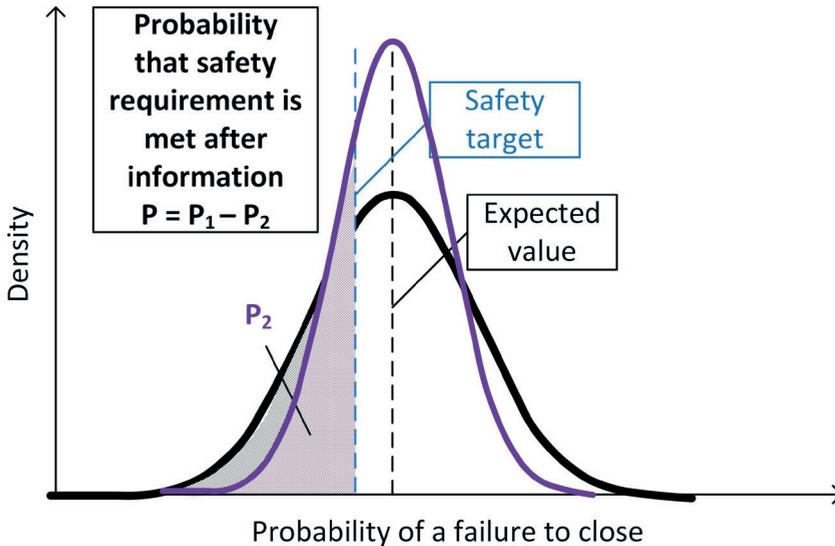
**Figure 5.8:** Proposed correction  $P_2$  for remaining uncertainty after implementation of the model refinement. The uncertainty around the probability of a failure to close before and after reducing uncertainty is described by a (normal) probabilistic distribution. The remaining uncertainty is described by a narrower distribution with the same expected value.
