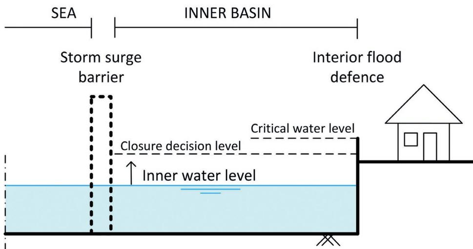
**Figure 2.1:** Schematic cross-section indicating the elements of a storm surge barrier flood protection system. A storm surge barrier is open in normal conditions and, therefore, indicated with a dotted line. At the interior flood defence, the critical water level is assumed to be equal to the crest level for visual clarity. The closure decision level is below the critical water level to account for water level forecast errors, the river gradient and local wind set-up.
