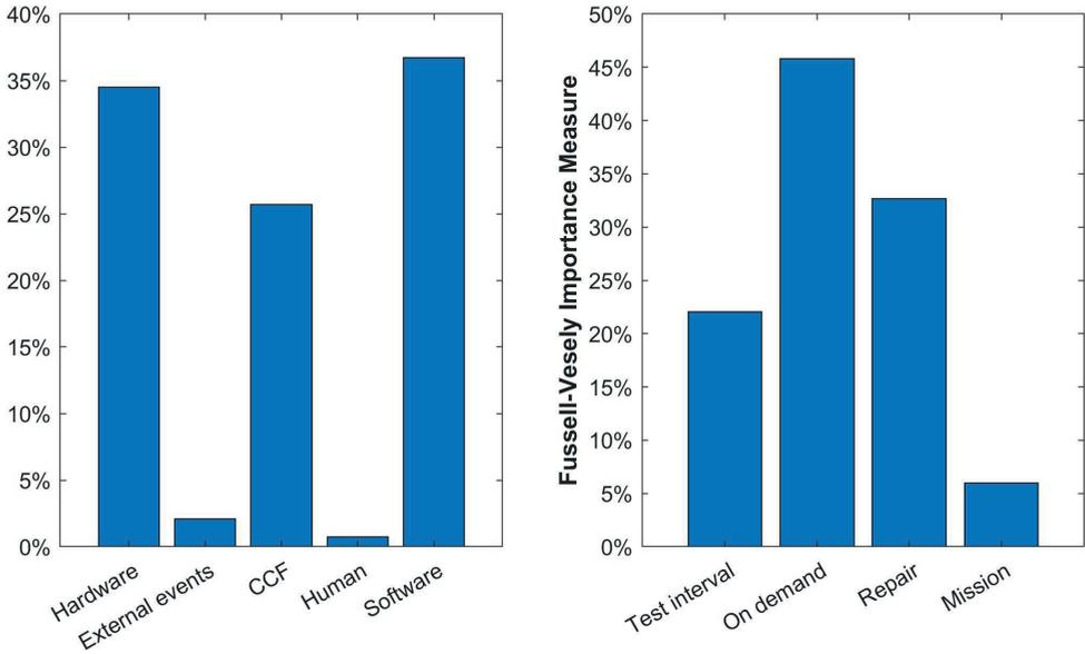
**Figure 4.5:** Fussell-Vesely importance of failure categories (left) and unavailability types (right) of the Maeslant barrier case study
