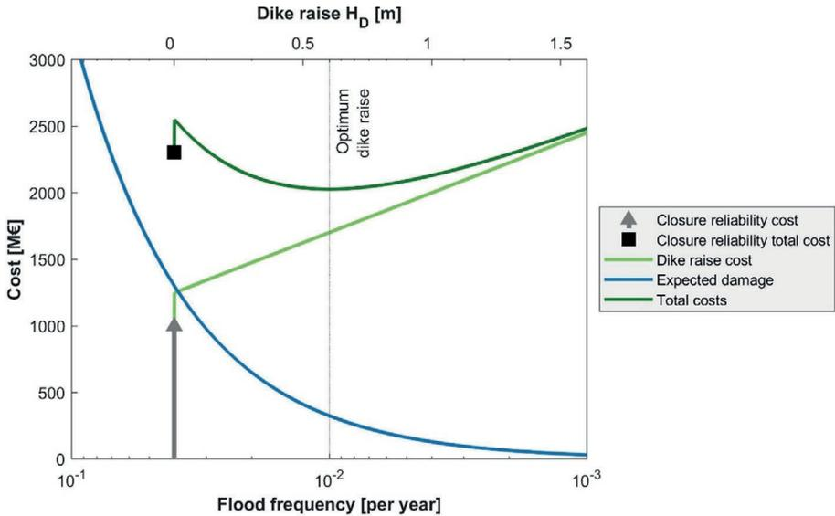
**Figure 3.5:** Optimization with storm surge barrier improvement. Dike raise parameters are the same as the previous figure. Storm barrier improvement with a cost of 1000 M€ has a probability of non-closure of 4/100 requests. The optimal solution is to combine this improvement with a dike raise of 0.6 meter, resulting in a flood frequency of 1/100 years.
