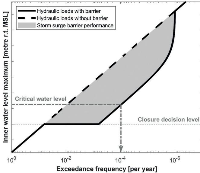
**Figure 2:** Schematic relations of exceedance frequencies of extreme water level maxima with and without a storm surge barrier based on the Maeslant barrier (Rotterdam, Netherlands), aiming at explaining the concept of “storm surge barrier performance”. The method and case study describe how the hydraulic loads with a barrier are developed. Figure 2.12 presents how barrier failure mechanisms contribute to these hydraulic loads.
