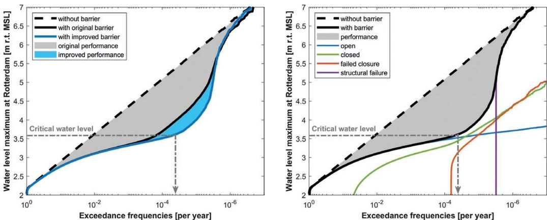
**Figure 2.15:** Exceedance frequencies with a performance improvement, which has lowered the probability of failed closure from 1/100 to 1/1000 on demand. Differences in performance for frequencies below  $10^{-6}$  per year are caused by the inaccuracy of the Monte Carlo Simulation for lower frequencies.
