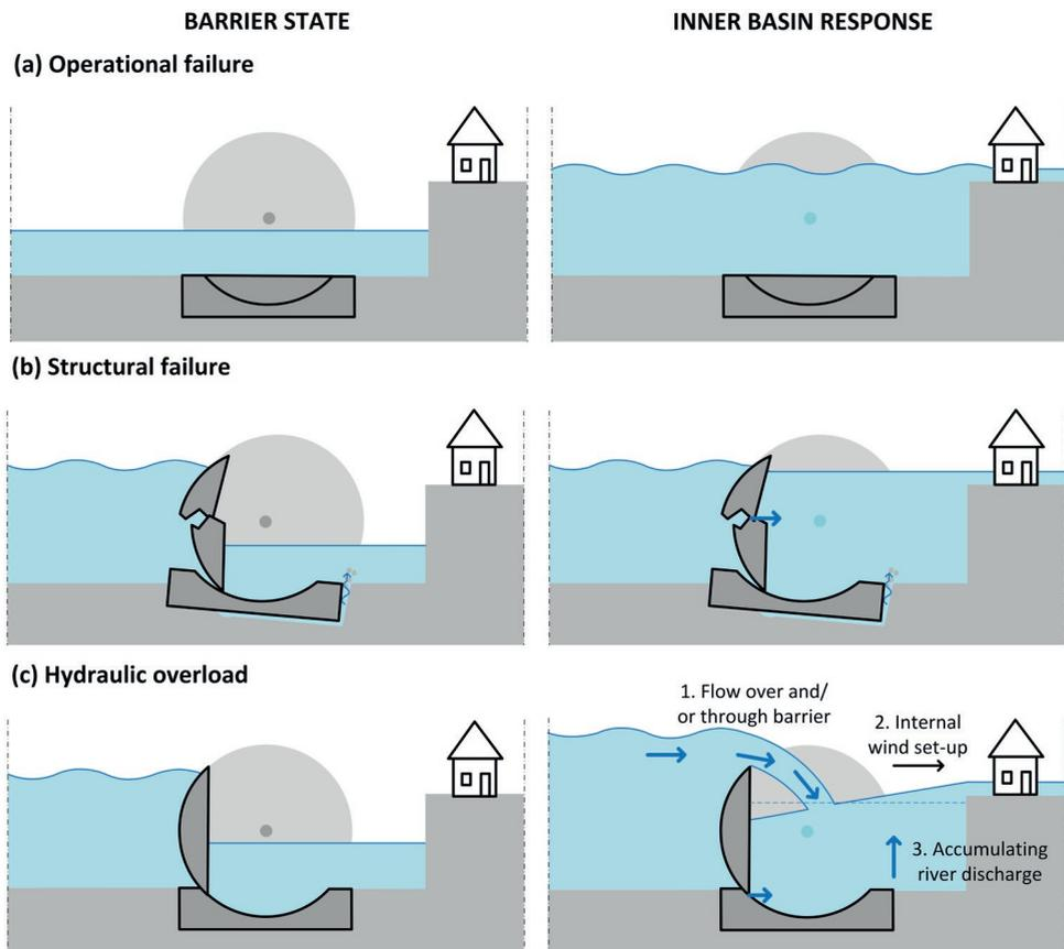
**Figure 1.3:** Principal system failure mechanisms. The left figure presents the barrier (failure) mode, while the right figure shows the corresponding inner basin response, which leads to exceedance of the critical water level.
