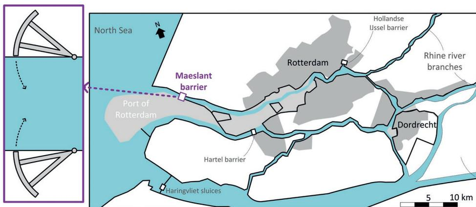
**Figure 2.9:** Schematic map with top view of the Maeslant barrier (left) and region protected by this barrier (right). Urban areas are hatched dark grey, port areas light grey. Solid black lines are used to indicate flood defenses.
