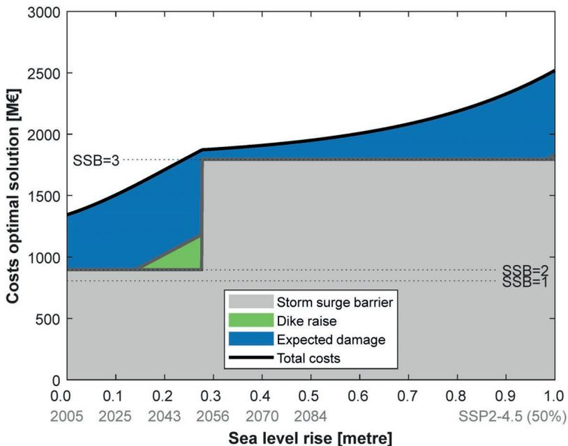
**Figure 3.9:** Total costs of optimal solutions with increasing sea level rise. The grey, green, and blue hatched areas indicate the storm surge barrier improvement costs, dike raise, and expected flood damage, respectively. The costs of the three storm surge barrier improvements are indicated with a dotted line. At the horizontal axis, the year corresponding to the amount of sea level rise according to scenario SSP2-4.5 (50%) is mentioned.
