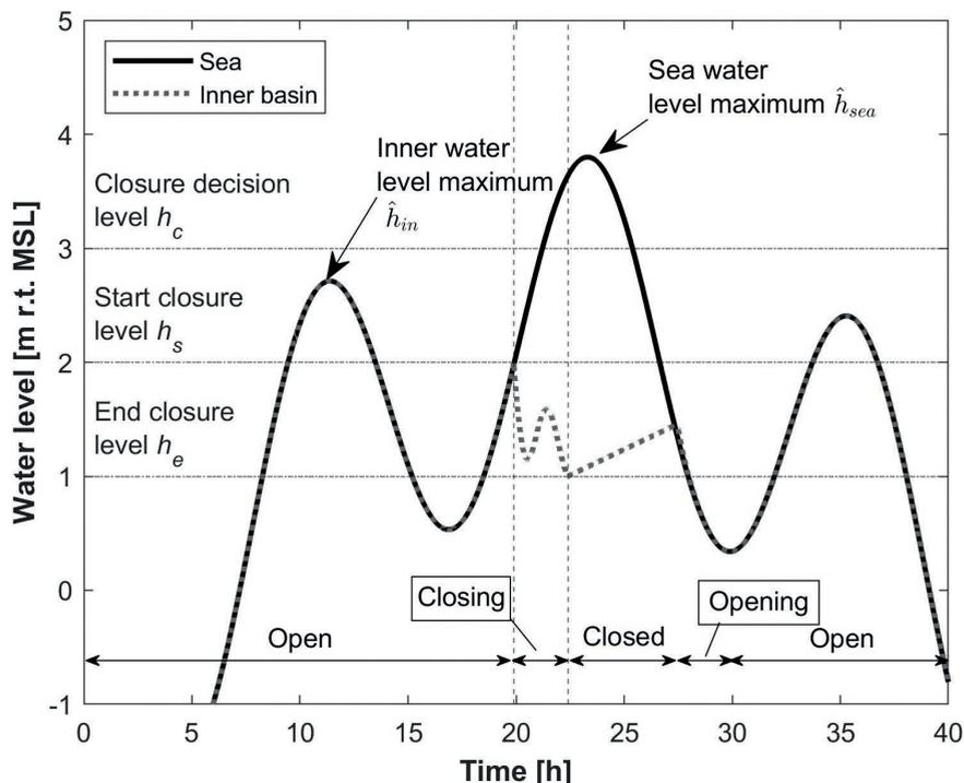
**Figure 2.4:** Example of inner and sea water levels during a closure procedure, based on the Maeslant barrier (Rotterdam, Netherlands). Water levels are expressed in meters relative to mean sea level (MSL).
