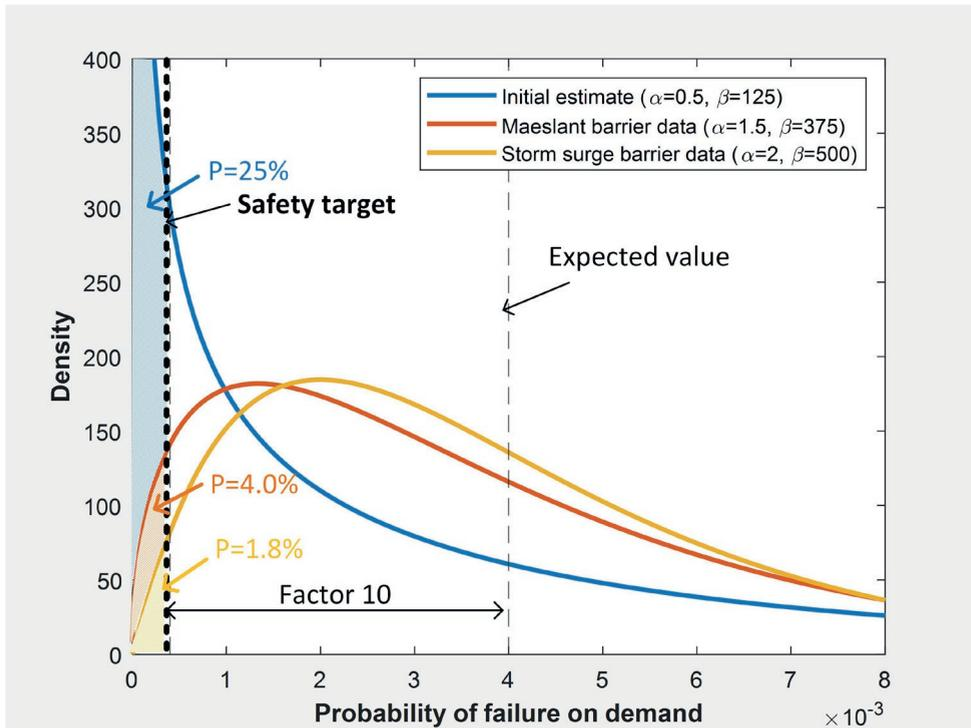
**Figure 5.10:** The probability distributions describing the uncertainty around the probability of a failure to close estimate for 1) initial estimate, 2) using Maeslant barrier data, and 3) using data from more storm surge barriers. The hatched areas indicate probabilities that the model input refinement reveals that the safety target is met.
