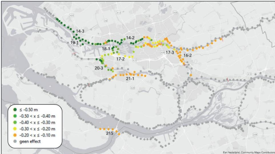
**Figure 3.11:** Effect of double barrier on extreme water level maxima with a frequency corresponding to legislated flood frequencies of interior flood defenses (Rijkswaterstaat, 2023)
