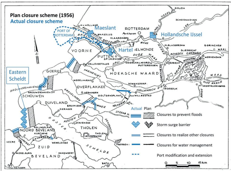
**Figure 1.5:** Schematic Deltaplan (Delta Committee, 1960) adapted in blue to indicate actual closure scheme. The Hollandsche IJssel barrier was the only storm surge barrier initially considered in the plan. It is constructed at the location indicated by the Delta Committee. The Deltaplan foresaw a closure dam at the Eastern Scheldt and dike raise along the New Waterway & Hartel canal, while storm surge barriers were realized here
