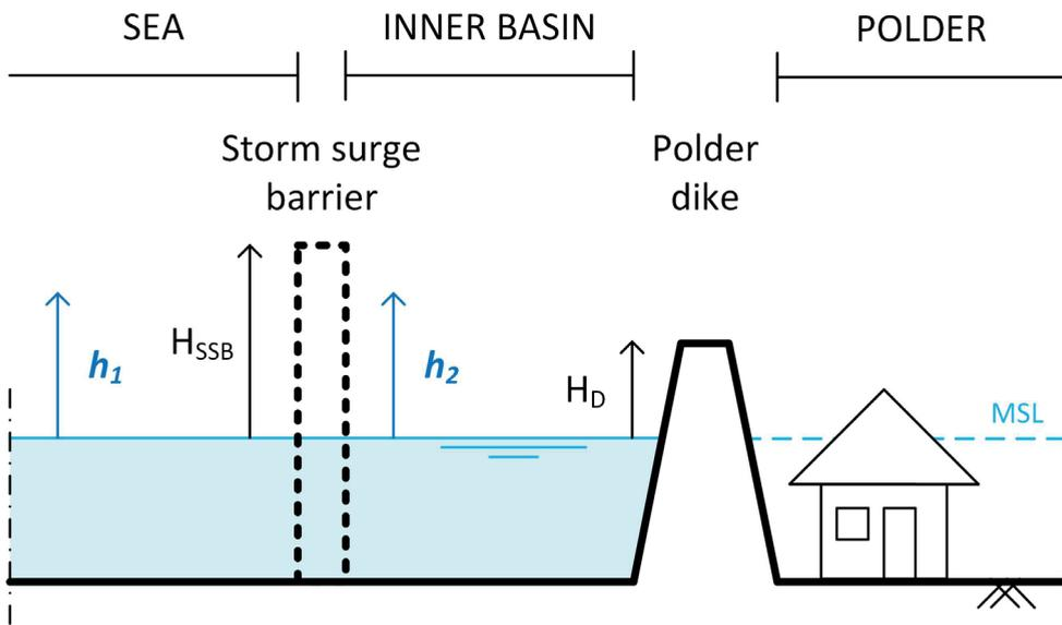
**Figure 3.3:** Schematic cross-section of a storm surge barrier flood protection system with one polder considered for the economic optimization model.
