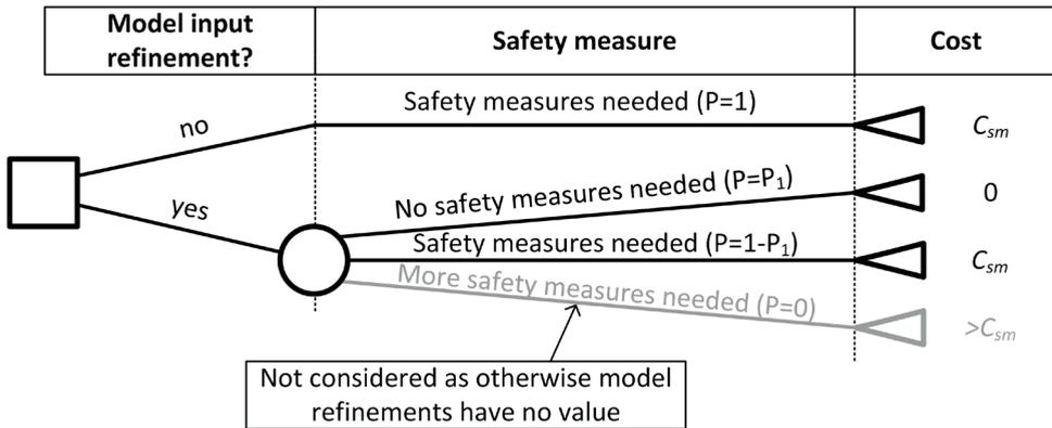
**Figure 5.5:** Decision tree of a model input refinement and its effects on the cost for safety target optimization. Costs of safety measures are described by the symbol  $C_{sm}$ , the probability that the model input refinement will reveal that no safety measures are needed  $P_1$ .
