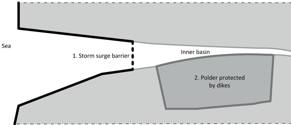
**Figure 3.2:** Schematic overview of a storm surge barrier flood protection system with one polder considered for the economic optimization model.
