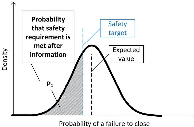
**Figure 5.7:** The probability that the safety target is met and no safety measures are, thus, needed given the uncertainty around the probability of a failure to close
