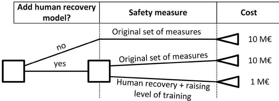
**Figure 5.4:** Decision tree of model refinement “human recovery model” and its effects on the cost for safety target optimization.
