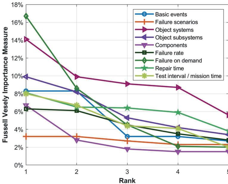
**Figure 4.6:** Fussell-Vesely importance of top 5 basic events, failure scenarios, elements of object decomposition and variables (failure rate, failure on demand, test interval, mission time and repair time) of the Maeslant barrier case study
