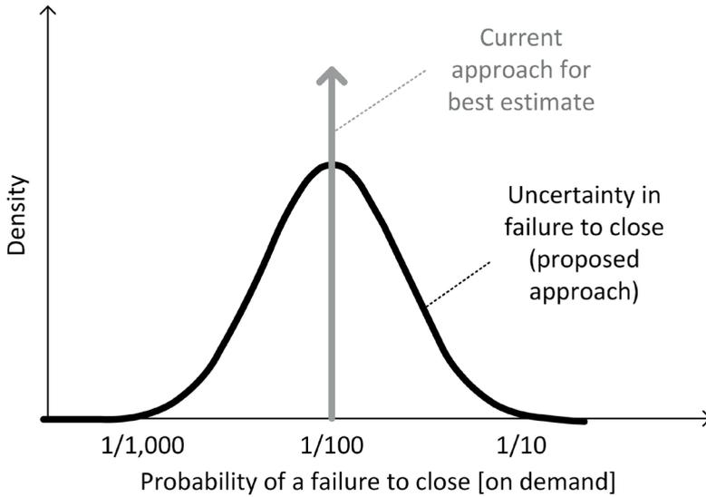
**Figure 5.6:** Current approach to describe failure probabilities at storm surge barrier and probabilistic distribution describing the uncertainty around the probability of a failure to close.
