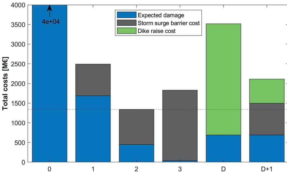
**Figure 3.8:** Total costs for selected solutions of Maeslant barrier case. The blue, grey, and green costs correspond with the risk, storm surge barrier costs, and dike raise costs, respectively. With a dashed line, the minimum total costs are indicated. The selected solutions are: 0) no measure, 1) single barrier without redundancies, 2) single barrier with redundancies, 3) double barrier, D) 1.4 meter dike raise and D+1) 0.3 meter dike raise with a single barrier without redundancies.
