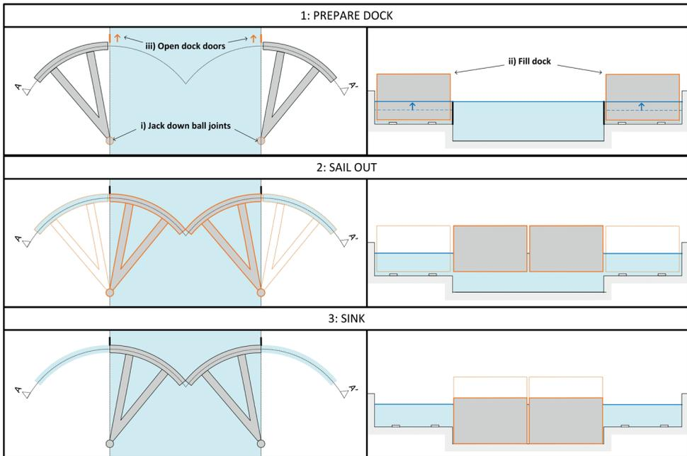
**Figure 1.6:** Schematic top view (left) and cross-section (right) of floating sector arms during three main closure procedure steps. Orange solid lines highlight gate parts that have moved during the main closure steps, and orange dotted lines indicate where the gate part was positioned in the previous step.
