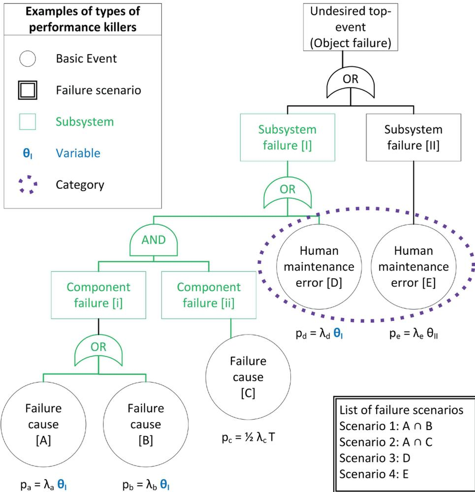
**Figure 4.1:** Example fault tree of an object with two subsystems of which one has two components. The fault tree aims to illustrate that even for a relatively simple system, there are many performance killers of which five examples are highlighted: any basic event, any failure scenario, subsystem A, repair time  $\theta_i$  and human maintenance errors.
