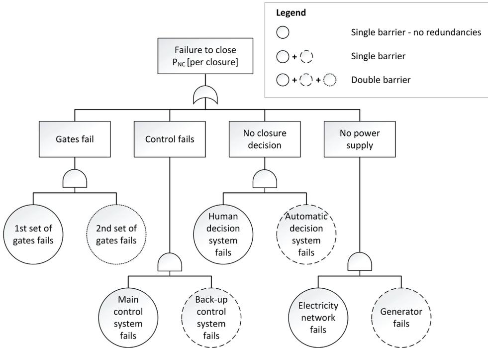
**Figure 3.7:** Simplified fault tree proposed for Maeslant barrier case. Basic events belonging to all storm surge barrier arrangements are indicated with solid borders. Basic events corresponding to a single and double barrier have dashed borders. The double barrier has an added basic event with a dotted border.
