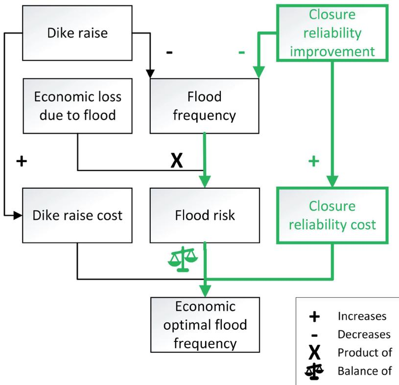
**Figure 3.1:** Process to find economic optimal flood frequencies. In black, the principle of the model of van Dantzig (1956) is shown. In green, the addition proposed by this chapter is indicated.
