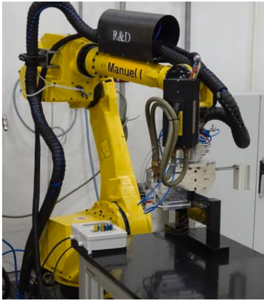
Fig. 2. Conduction welding robot at Fokker/GKN Aerospace.
