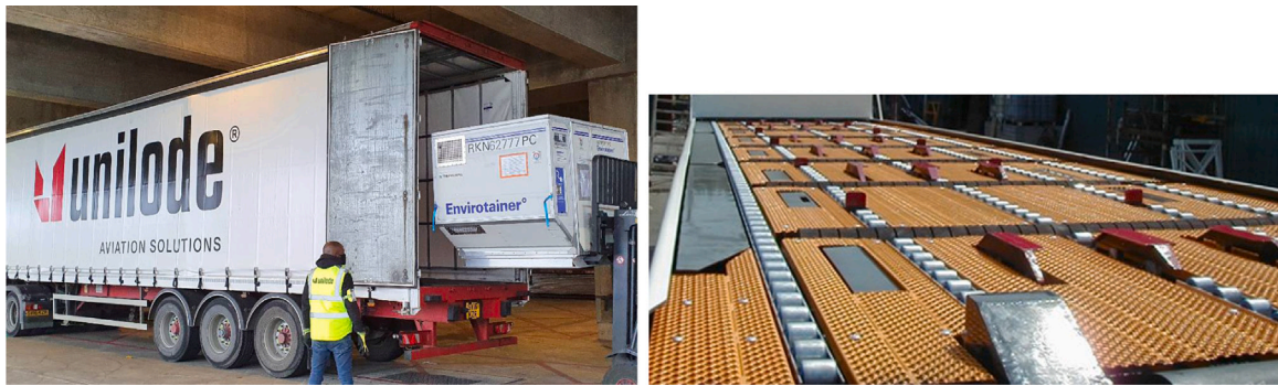
Fig. 2. Unloading of a ULD from a trailer (left) and focus on the trailer's base with blocks and guides (right). From https://www.stattimes.com and https://www.jbtc.com respectively. Potentially, trailers may be accessible from the side thanks to removable covers (Fig. 2(a)). However, blocks and guides (Fig. 2(b)) impose that the forklifts can only unload ULDs following a LIFO sequence.
