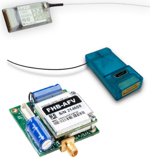
(a) The suggested configuration of a Remote ID receiver, GNSS ADS-B and satellite transmitter-receiver
