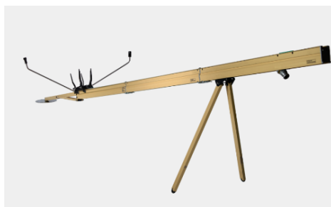
(a) PL-40 pneumatic catapult that will be used to launch the Puffin
