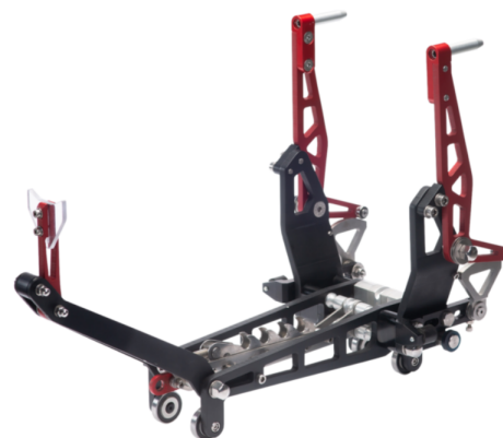
(b) Customised carriage to be mounted to the catapult that will be designed to specifically carry the Puffin
