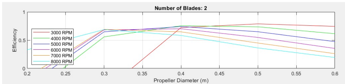
Figure 7.4: Propeller efficiency vs diameter for various RPM, for estimated required diameter the propeller efficiency is 0.7, the efficiencies increase with decreasing rpm and increase with the increasing diameter. Increasing the diameter is to be avoided for impact performance.
