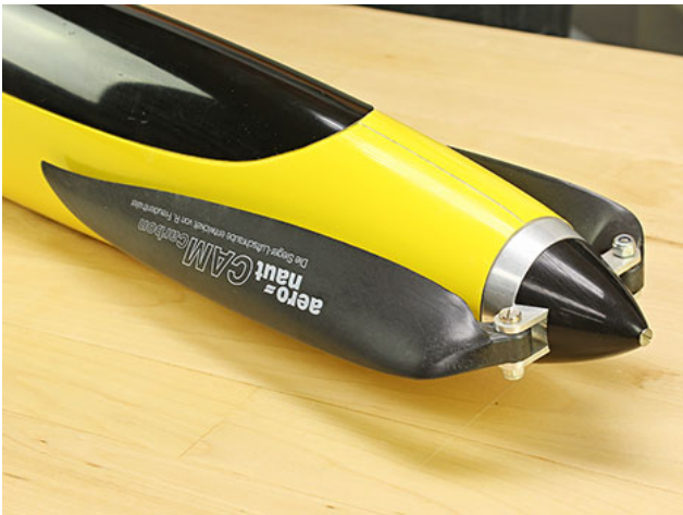
(a) The blades folded onto the fuselage, mounted to the adapter.
