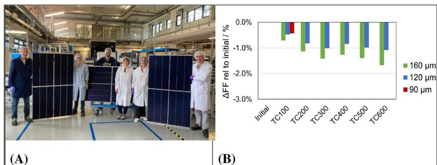
**FIGURE 11** (A) 60-M2 cell equivalent SHJ shingled modules using 12 strings of 32 cut-cells and a glass-glass design. Source: CEA. (B) Evolution of  $\Delta FF$  after TC for SHJ shingle modules integrating different wafer thicknesses; 90  $\mu\text{m}$  configuration is currently still going through further extensive TC tests. Source: CEA<sup>31</sup> [Colour figure can be viewed at [wileyonlinelibrary.com](http://wileyonlinelibrary.com)]
