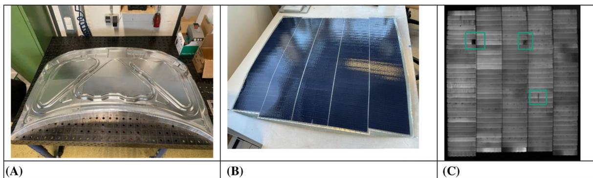
**FIGURE 14** (A) Aluminum form for the lamination process, (B) picture of a reduced-size VIPV module with five shingle string, and (C) electroluminescence (EL) image of the VIPV module after lamination, before the vibration testing [Colour figure can be viewed at [wileyonlinelibrary.com](http://wileyonlinelibrary.com)]
