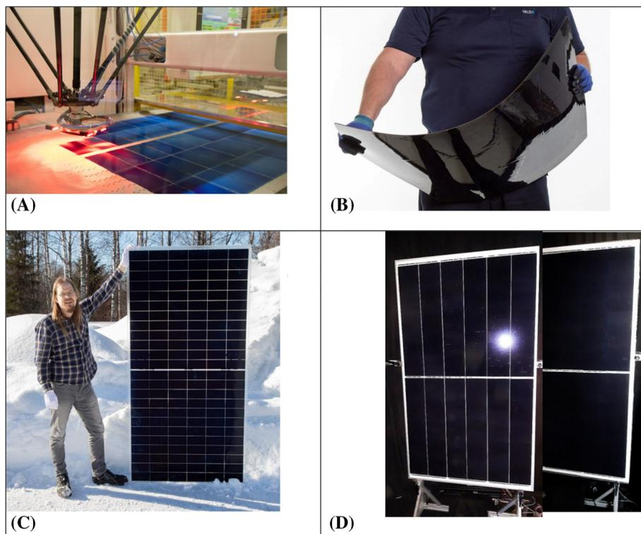
**FIGURE 9** (A) High speed delta robot in HAMA line. Source: Valoe. (B) Flexible odd form IBC module for VIPV application. Source: Valoe. (C) Bifacial glass-glass Chrystal Twin module with 144 IBC half-cut. Source: Valoe. (D) Monofacial glass-backsheet modules from IBC using either gapless strings (left) or a fully gapless (right) design. Source: ISC<sup>52</sup> [Colour figure can be viewed at [wileyonlinelibrary.com](https://onlinelibrary.wiley.com/doi/10.1002/pip.3667)]
