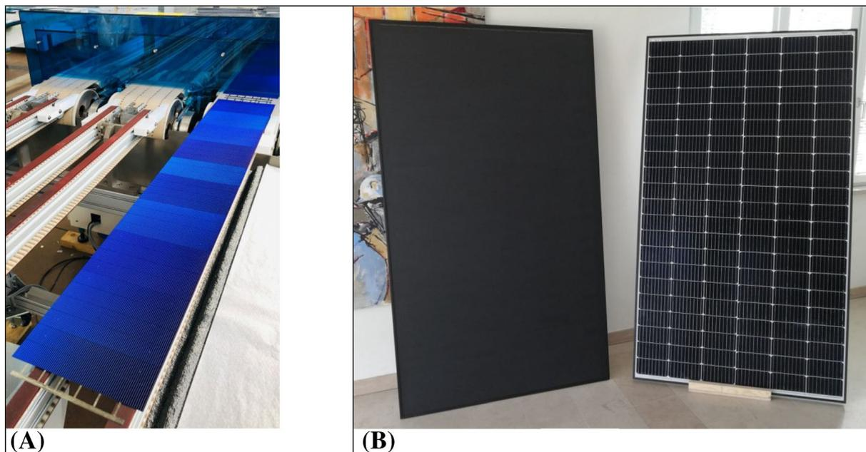
**FIGURE 8** (A) Finished string of 39 full size SHJ shingles with the string ribbons also attached in the applied Sonetto™ tool. Source: AMAT. (B) Left: Shingle full black module with 4 mm thick glass for BIPV, right: reference Tarka 120 module with 9BB design. Source: Voltec Solar [Colour figure can be viewed at [wileyonlinelibrary.com](http://wileyonlinelibrary.com)]
