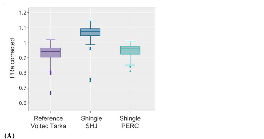
**FIGURE 18** (A) Average PRa corrected for temperature for systems installed at CEA in Cadarache. (B) Monthly PRa corrected for temperature for shingle SHJ bifacial module installed in CSEM/EPFL, UL, and ISC [Colour figure can be viewed at [wileyonlinelibrary.com](http://wileyonlinelibrary.com)]
