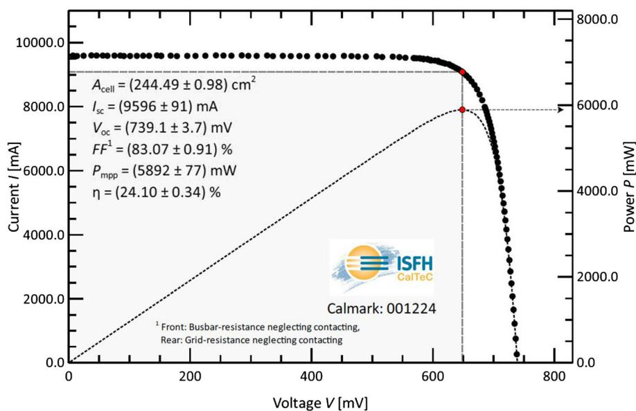
**FIGURE 4** Externally confirmed efficiency of 24.1% for a full area M2-size (area = 244.5 cm<sup>2</sup>) SHJ cell with a shingle metallization layout produced at CEA-INES pilot-line in 2021 [Colour figure can be viewed at [wileyonlinelibrary.com](http://wileyonlinelibrary.com)]
