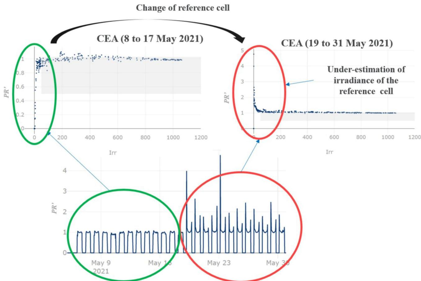
**FIGURE 19** Top graphs:  $PR_{a}$  corrected by temperature versus irradiance for the string of 10 benchmark modules Tarka-120 measured in Cadarache, bottom graph:  $PR_{a}$  corrected by temperature between May 8 and 31, 2021 [Colour figure can be viewed at [wileyonlinelibrary.com](https://onlinelibrary.wiley.com/doi/10.1002/ep.3667)]
