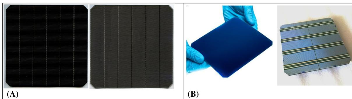
**FIGURE 2** (A) M2-size SHJ cell with a six-segment shingle metallization layout at the front (left image) and rear (right image) sides and (B) M2-size ZEBRA IBC solar cell with no metallization at the front (left image) and a  $2 \times 4$  busbars ( $2 \times 4$ BB) half-cut layout at the rear (right image). [Colour figure can be viewed at [wileyonlinelibrary.com](https://onlinelibrary.wiley.com/doi/10.1002/pip.3667)]
