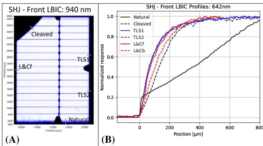
**FIGURE 6** (A) LBIC image of SHJ cell cut using mechanically cleaving, laser scribe and cut (L&C), and thermal laser separation (TLS). Source: Bokalic et al.<sup>40</sup> (B) LBIC response across the cut edges for the different positions marked in (A). Source: Bokalic et al.<sup>40</sup> [Colour figure can be viewed at [wileyonlinelibrary.com](https://onlinelibrary.wiley.com)]
