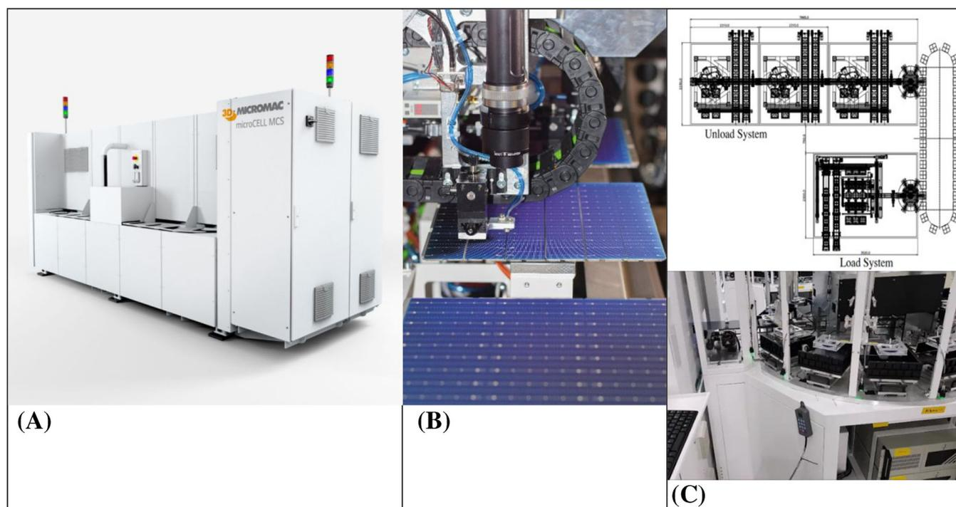
**FIGURE 7** (A) microCELL™ MCS high-throughput shingling tool developed by 3D-Micromac in HighLite, (B) view of one of the process station, (C) top: schematic of automatic system for standalone operation of the microCELL™ MCS with high-throughput loading of full wafers and unloading of shingles into dedicated trays, bottom: partial view of the loading system [Colour figure can be viewed at [wileyonlinelibrary.com](http://wileyonlinelibrary.com)]
