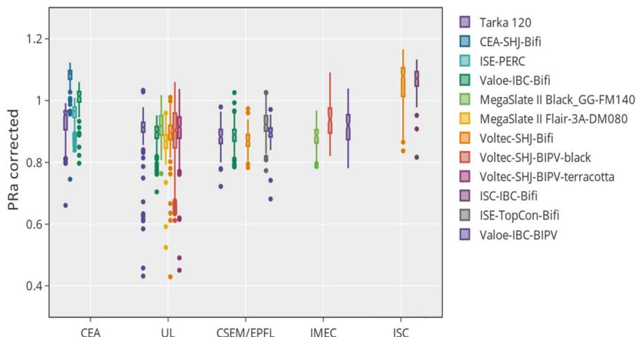
**FIGURE 17** Box-plot of the monthly performance ratio of the array corrected for temperature (PRa\_corrected or PRa\_corr in short) for the different module types and locations [Colour figure can be viewed at [wileyonlinelibrary.com](http://wileyonlinelibrary.com)]
