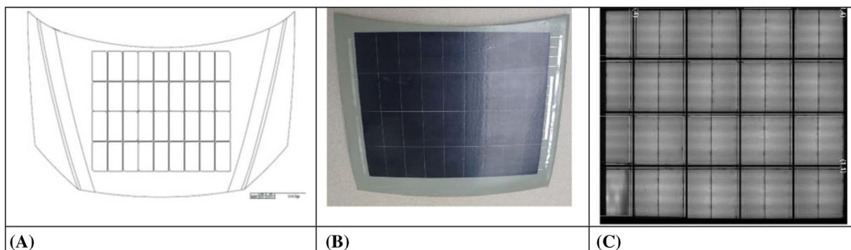
**FIGURE 13** (A) Layout of the IBC cut cells on the VIPV demonstrator car bonnet, (B) picture of reduced-size VIPV module, and (C) electroluminescence (EL) image of the VW Polo VIPV demonstrator taken after lamination and before the vibration testing. *Source:* ISFH [Colour figure can be viewed at [wileyonlinelibrary.com](http://wileyonlinelibrary.com)]
