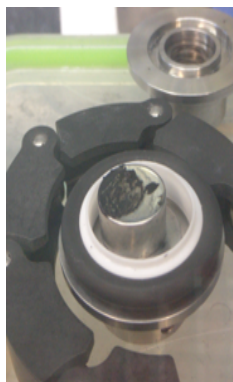
Figure 5.6: Electrolyte decomposition residue in NaAlg 2w% aq. system
