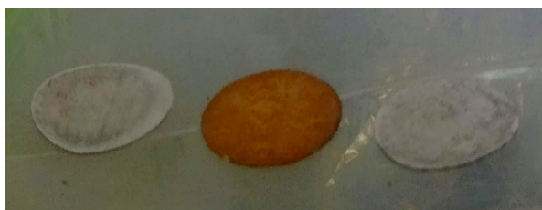
Figure 4.2: Formation of white LiOH on Li foil on prolonged contact with LiAlg
