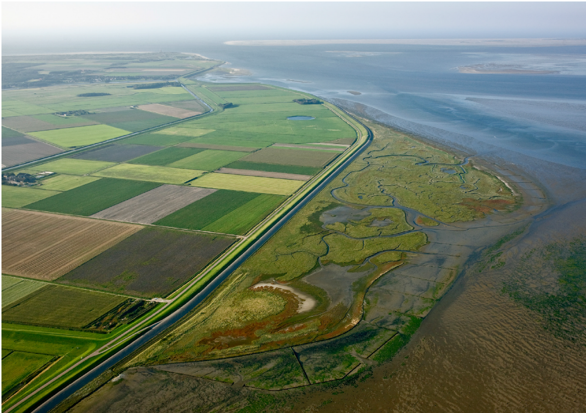
Figure 1.2: De Schorren, Texel. This salt marsh is currently a nature reserve. The dike separates the salt marsh from the protected hinterland. Several groyne structures can be seen at the edges (photo from Living Dikes archive).
