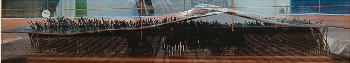
Figure 2.5: A small plate of modeled vegetation (mimics) used in experiment representing salt marsh vegetation. The vegetation moves with the waves. See also appendix A
