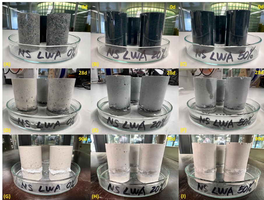
Fig. A2. Visual observation of efflorescence of NS-activated AAS mortars with time.
