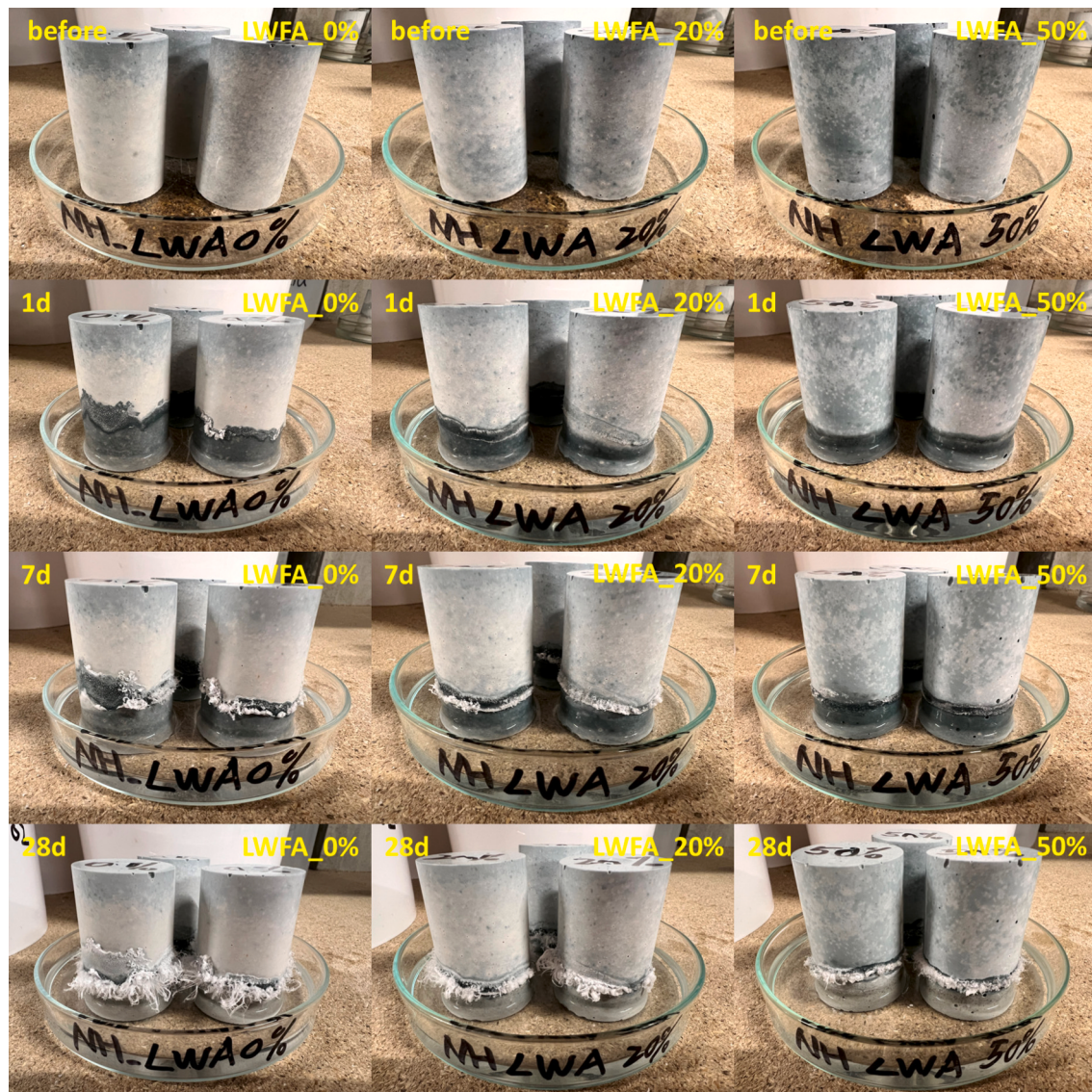
Fig. 3. Visual observation of the efflorescence of AAS mortar cylinders with time.
