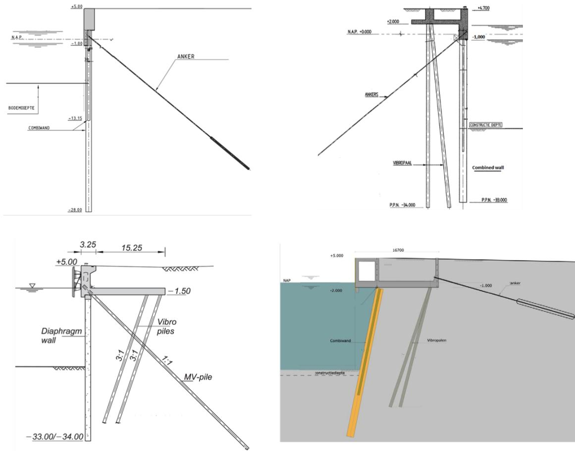
FIGURE 11.4: Amazonehaven southside (toleft), quay Brammen terminal (top right), Euromax (bottom left), Amazonehaven EMO5 (bottom right)
