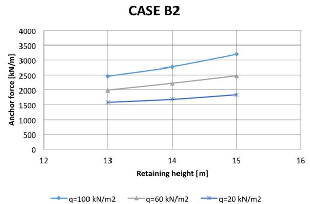
FIGURE 8.10: Maximum anchor forces CASE B2
