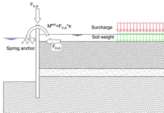
FIGURE 8.2: schematization of a deep-sea quay wall in D-sheet
