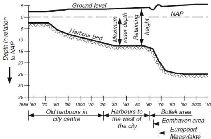
FIGURE 1.1: The increase of water depth and retaining height [1]
