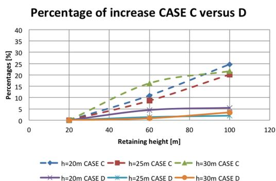
FIGURE 10.10: Increase of percentage by increasing surcharge for case C-D
