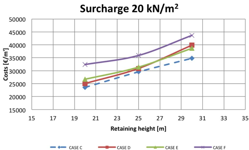
FIGURE 10.7: Construction costs for surcharge 20kN/m<sup>2</sup>
