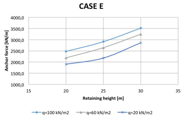
FIGURE 8.16: Maximum anchor forces CASE E
