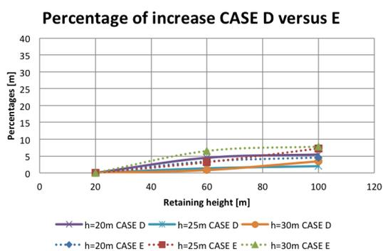
FIGURE 10.12: Increase of percentage by increasing surcharge for case D-E
