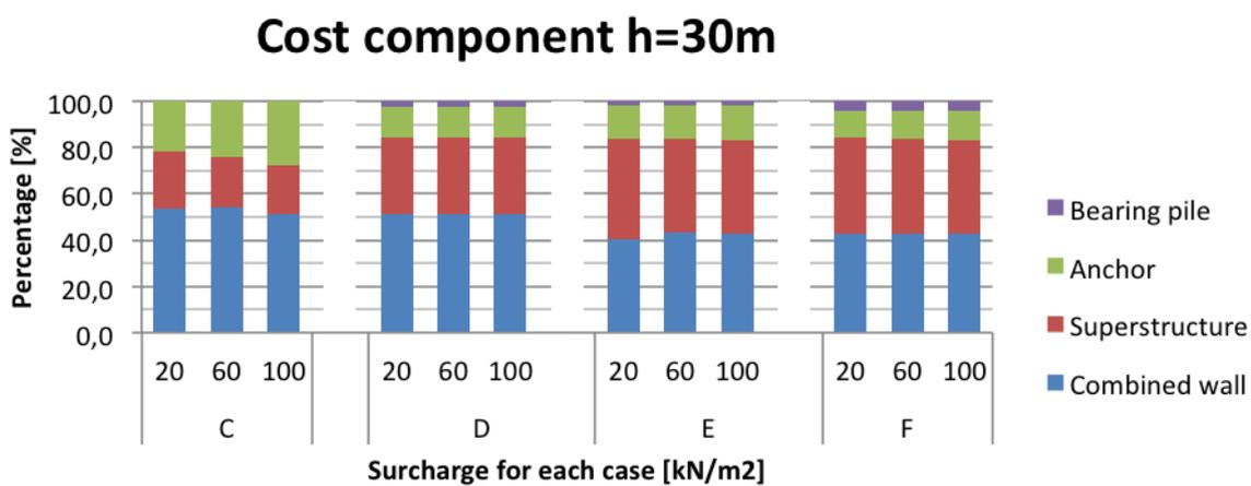
FIGURE 10.17: Cost components for retaining height 30m
