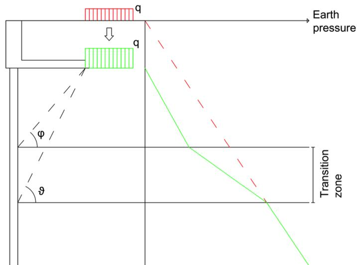
FIGURE 7.1: Principle of a relieving platform
