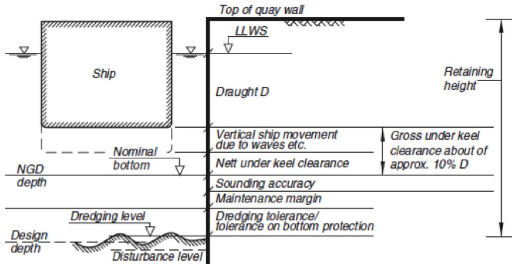
FIGURE 5.6: Important factors influencing the total retaining height[1]
