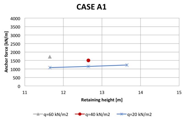
FIGURE 8.4: Maximum anchor forces CASE A1
