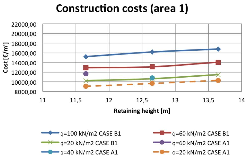
FIGURE 10.1: Construction costs for several design cases in area 1
