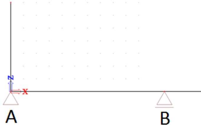
FIGURE 7.3: Static determined system
