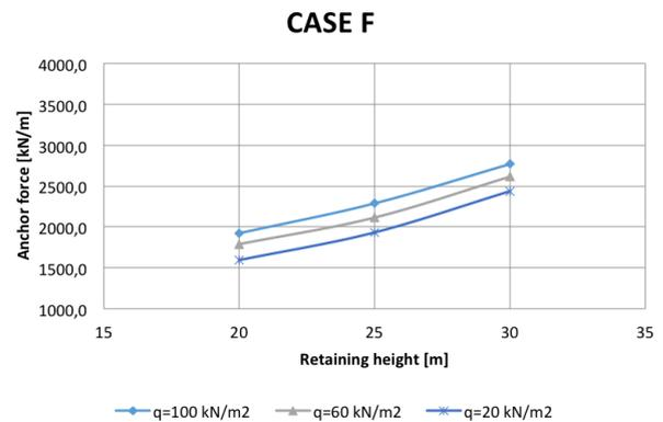
FIGURE 8.18: Maximum anchor forces CASE F
