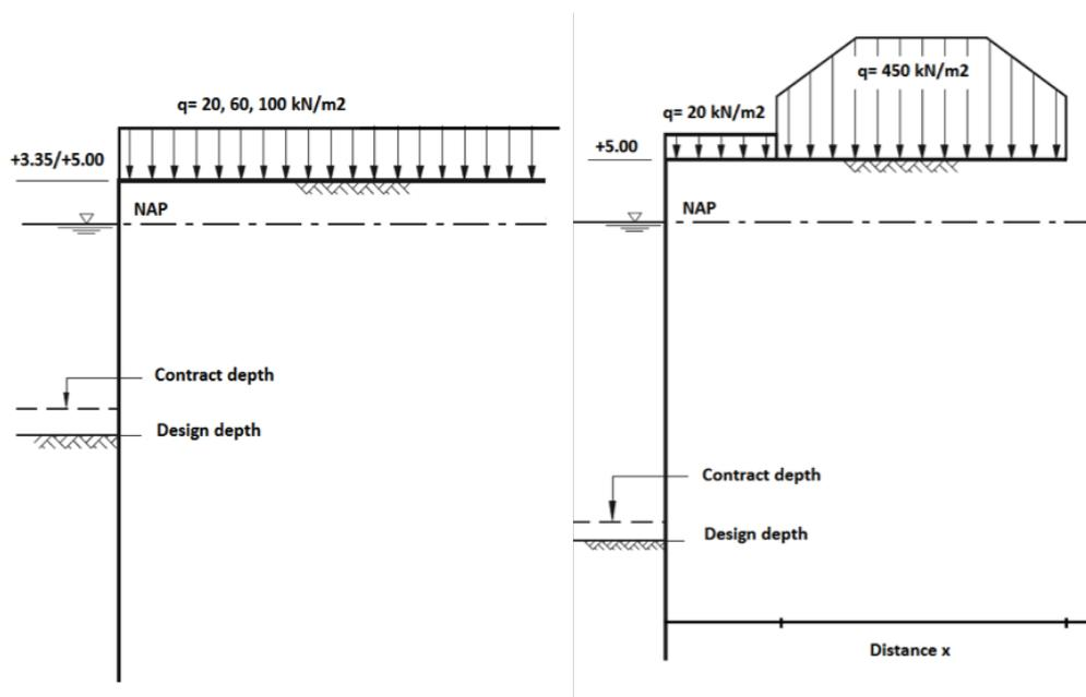
FIGURE 5.7: Schematization of surcharge loads
