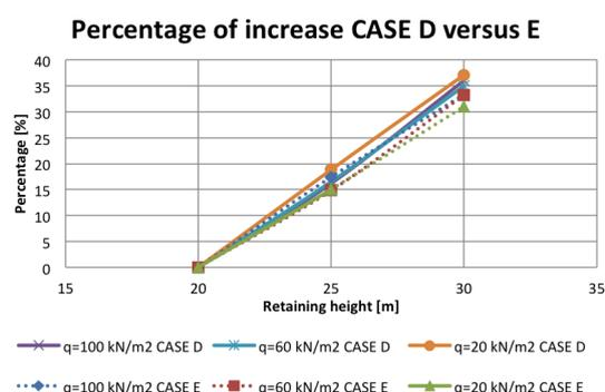
FIGURE 10.13: Increase of percentage by increasing retaining height for case D-E
