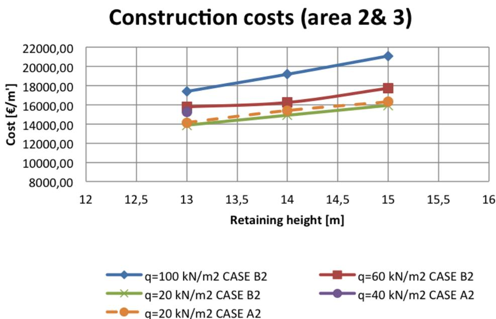
FIGURE 10.4: Construction costs for several design cases in area 2 &amp; 3
