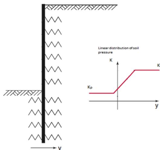
FIGURE 5.4: Interaction model used for the elastically supported beam
