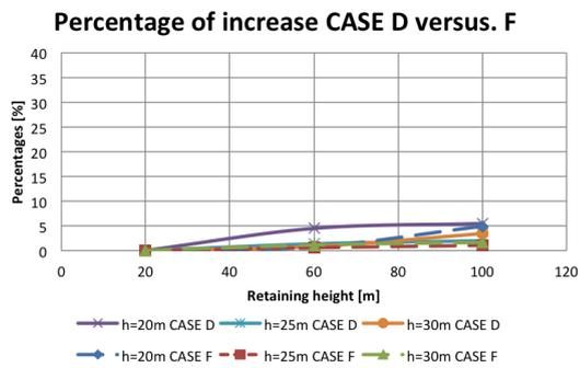
FIGURE 10.14: Increase of percentage by increasing retaining height for case D-F
