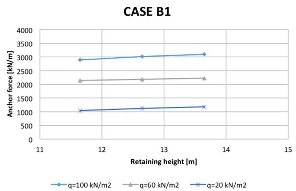
FIGURE 8.6: Maximum anchor forces CASE B1
