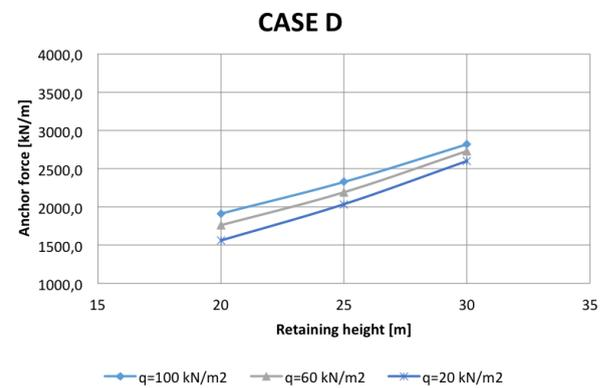
FIGURE 8.14: Maximum anchor forces CASE D
