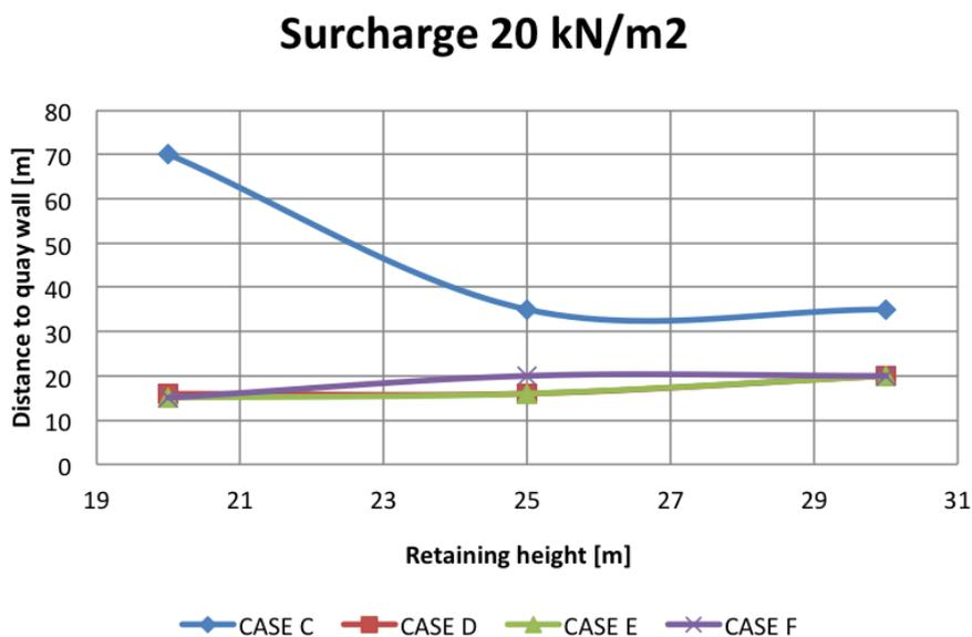
FIGURE 9.1: Minimum distance to the front of a quay wall, for surcharge  $20kN/m^2$
