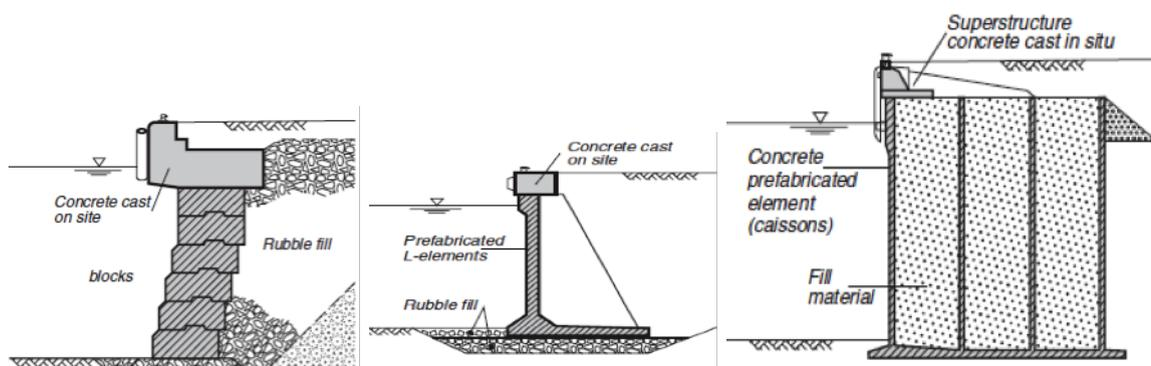
FIGURE 3.2: Principle of a block wall, an L-shaped wall and a caisson[1]
