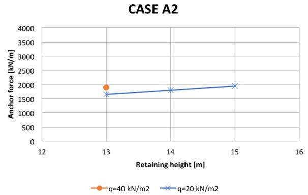
FIGURE 8.8: Maximum anchor forces CASE A2
