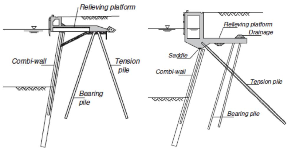
FIGURE 3.4: Principle of a structure with a high and low relieving platform[1]
