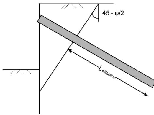
FIGURE 8.20: Principle of a MV-pile[1]
