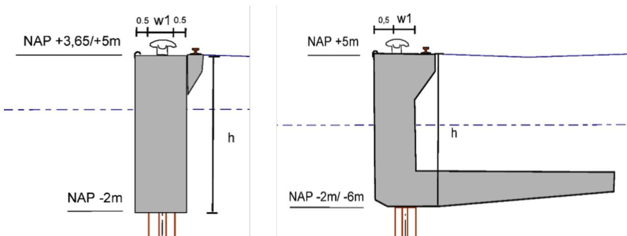
FIGURE 8.19: Cross-section superstructure
