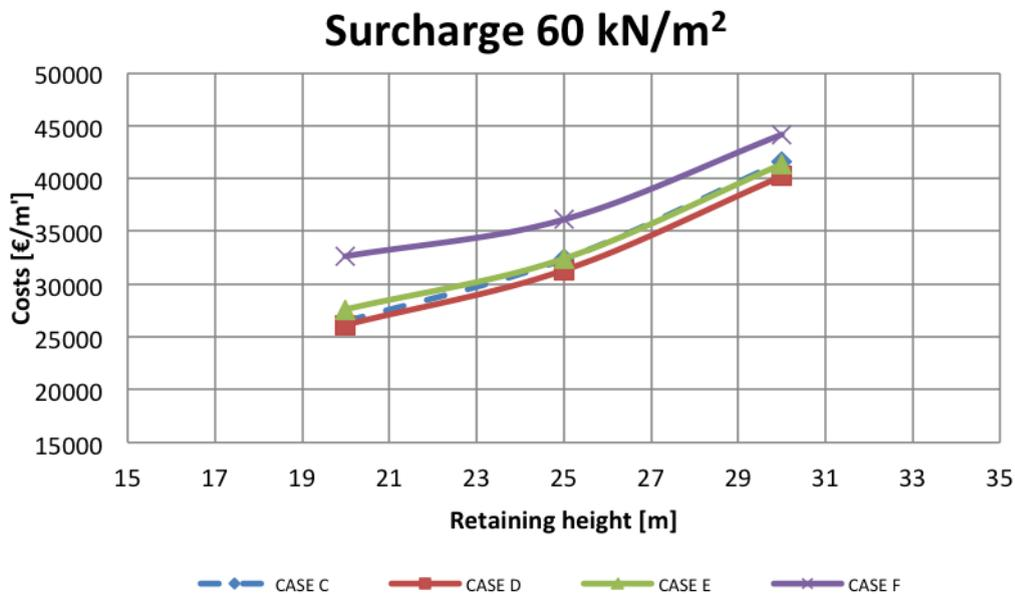
FIGURE 10.8: Construction costs for surcharge 60kN/m<sup>2</sup>
