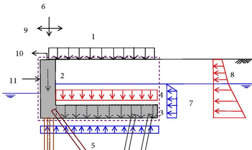
FIGURE 7.2: Loads acting on the relieving platform
