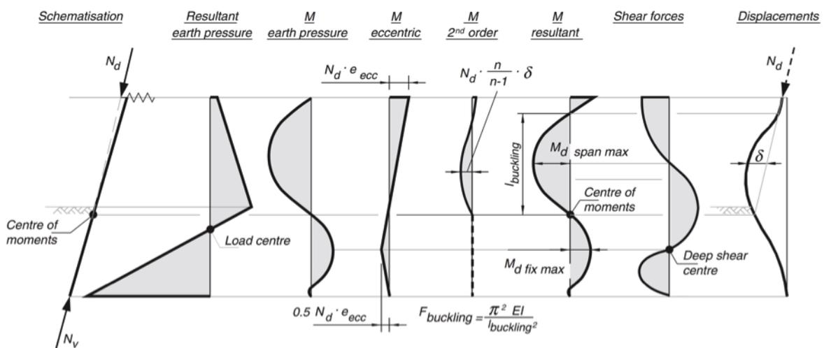
FIGURE 8.1: Principle of moment distribution[1]
