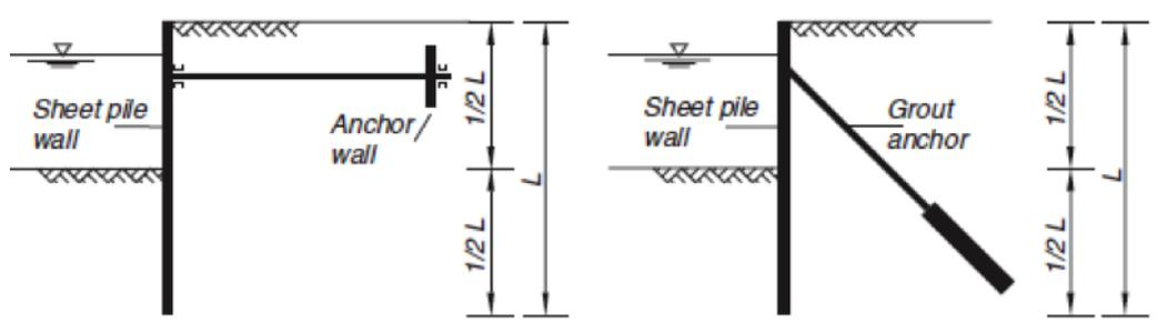
FIGURE 3.3: Principle of an anchored sheet pile wall[1]
