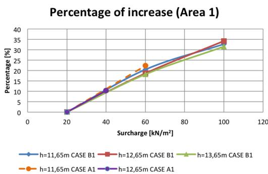
FIGURE 10.2: Increase of percentage by increasing surcharge in area 1
