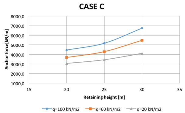
FIGURE 8.12: Maximum anchor forces CASE C
