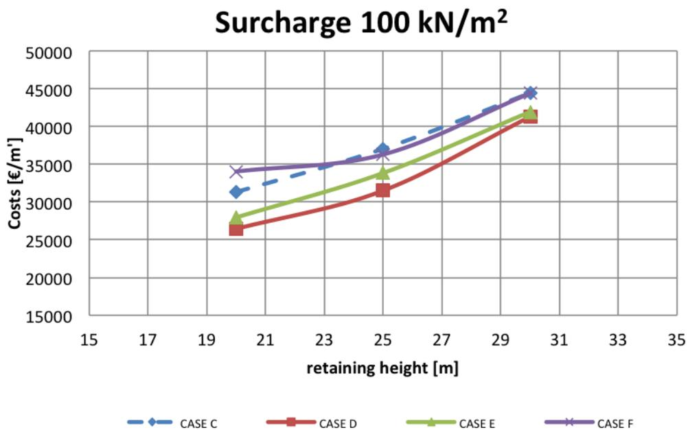
FIGURE 10.9: Construction costs for surcharge 100kN/m<sup>2</sup>
