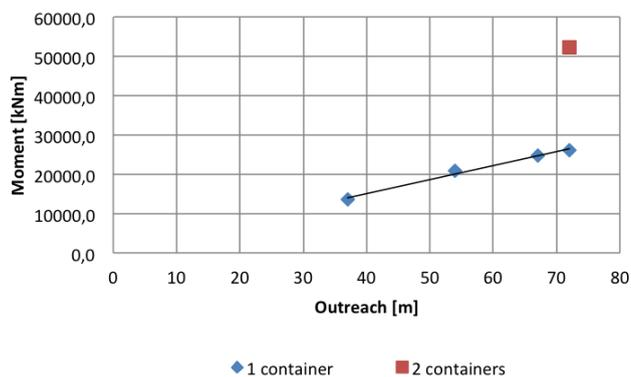
FIGURE 2.6: Increase outreach of cranes over time [17]
