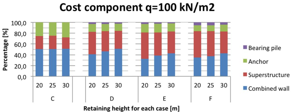
FIGURE 10.16: Cost components for surcharge 100kN/m<sup>2</sup>
