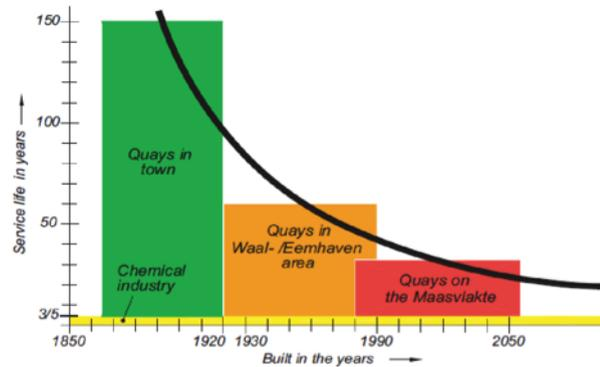
FIGURE 1.2: Decreasing of the functional use of quay walls Rotterdam [1]
