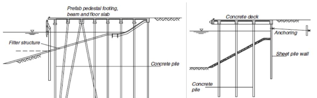
FIGURE 3.5: Principle of an open berth[1]
