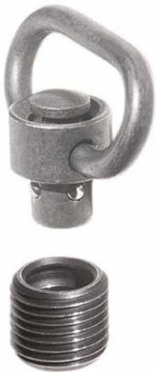
Figure X: By pushing the top button, the balls can fall in. Releasing the button the spring keeps the pin, and therefore the balls, in place, locking it in place.
