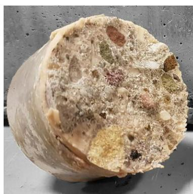
Figure 75: pulled off dolly: concrete failure at the surface of the concrete
