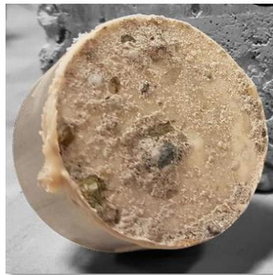
Figure 86: pulled off dolly sanded surface
