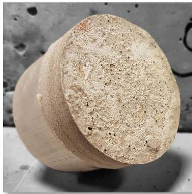
Figure 90: pulled off dolly sanded surface
