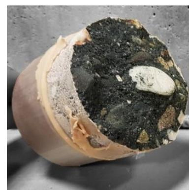
Figure 76: pulled off dolly: concrete failure at the tip of the drilled core
