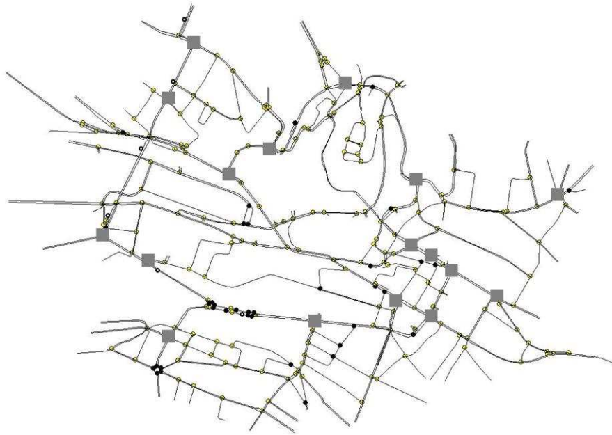
Figure 7 Lausanne network model with the 17 controlled intersections displayed as grey rectangles.
