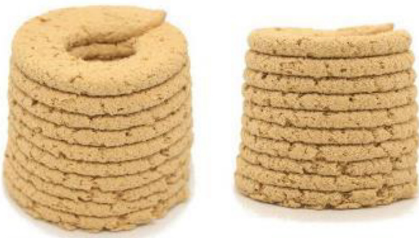
Figure 2 Tower for vertical shrinkage measurement
