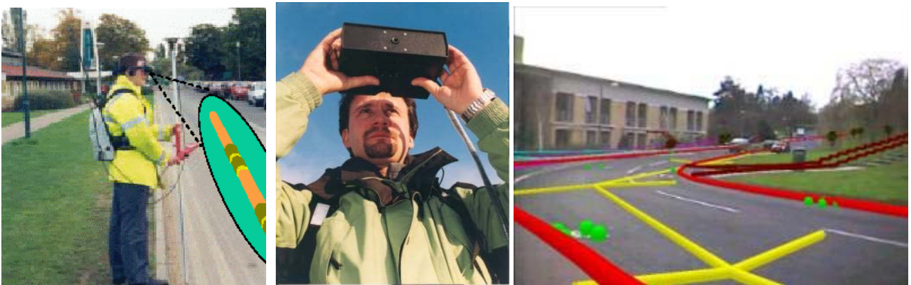
Figure 6-3: Subsurface Visualisation: HMD, virtual binoculars and a virtual view (University of Nottingham, IESSG)
