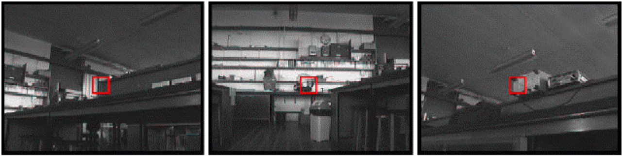
Figure 2-7: Automatically recognised and tracked templates (Davison 1999). Red squares indicate template content and its real-world position
