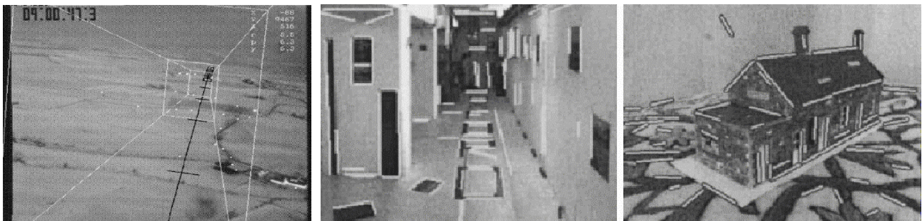
Figure 2-8 Point tracking, Harris 1992 (left), Line tracking, Schmid and Zisserman, 1997 (middle, right)
