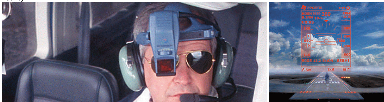
Figure 2-4: NOMAD retina scanning display (Microvision)
