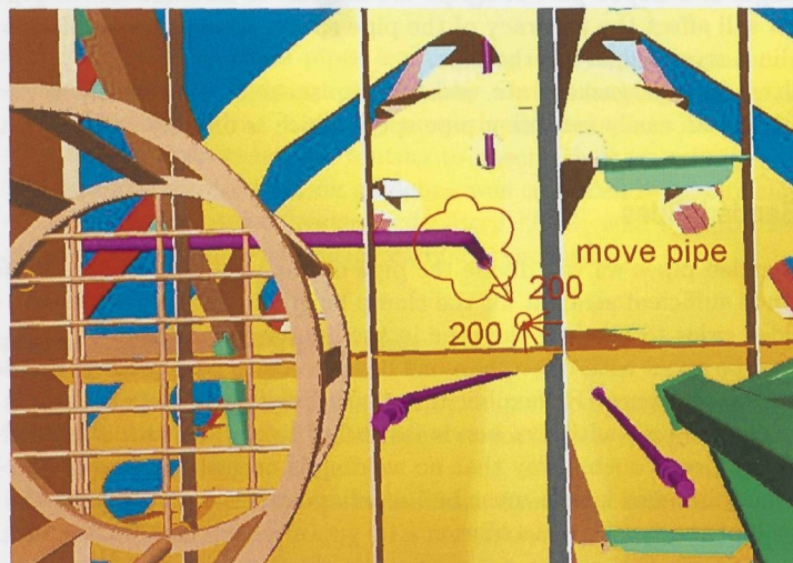
Figure 2.2: Pipe needs to be moved near the steel construction
