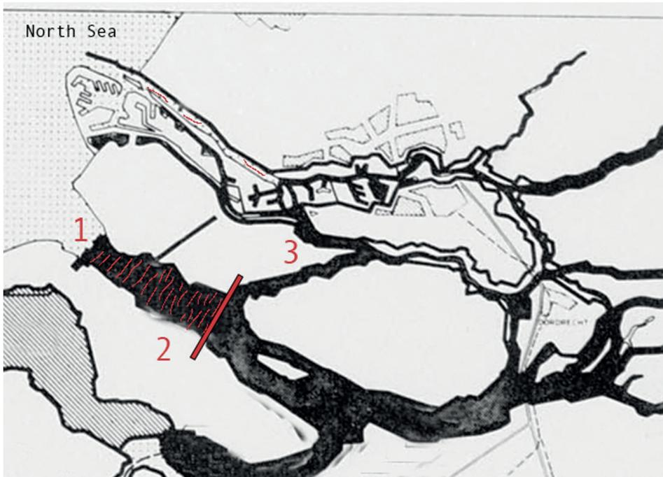
Figure 4. (1) The Haringvliet Dam. (2) In red, the negotiated saline threshold in the Haringvliet near the town of Middelharnis. (3) Spui waterway, risk of backward salt-water intrusion. Black parts represent fresh water, white/dotted parts saline water. CC BY- SA adapted map from Wikimedia Commons; original commissioner: House of Representatives, The Netherlands.
