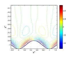
Contourplot of the residual horizontal flow for a sand wave with amplitude of 4 m in a depth H of 20 m and a maximum depth averaged flow velocity of  $0.5~{\rm ms}^{-1}$ . The dimensionless distance in the horizontal direction  $x^*$  and the vertical direction  $z^*$  is plotted on the x and z-axes, respectively.
