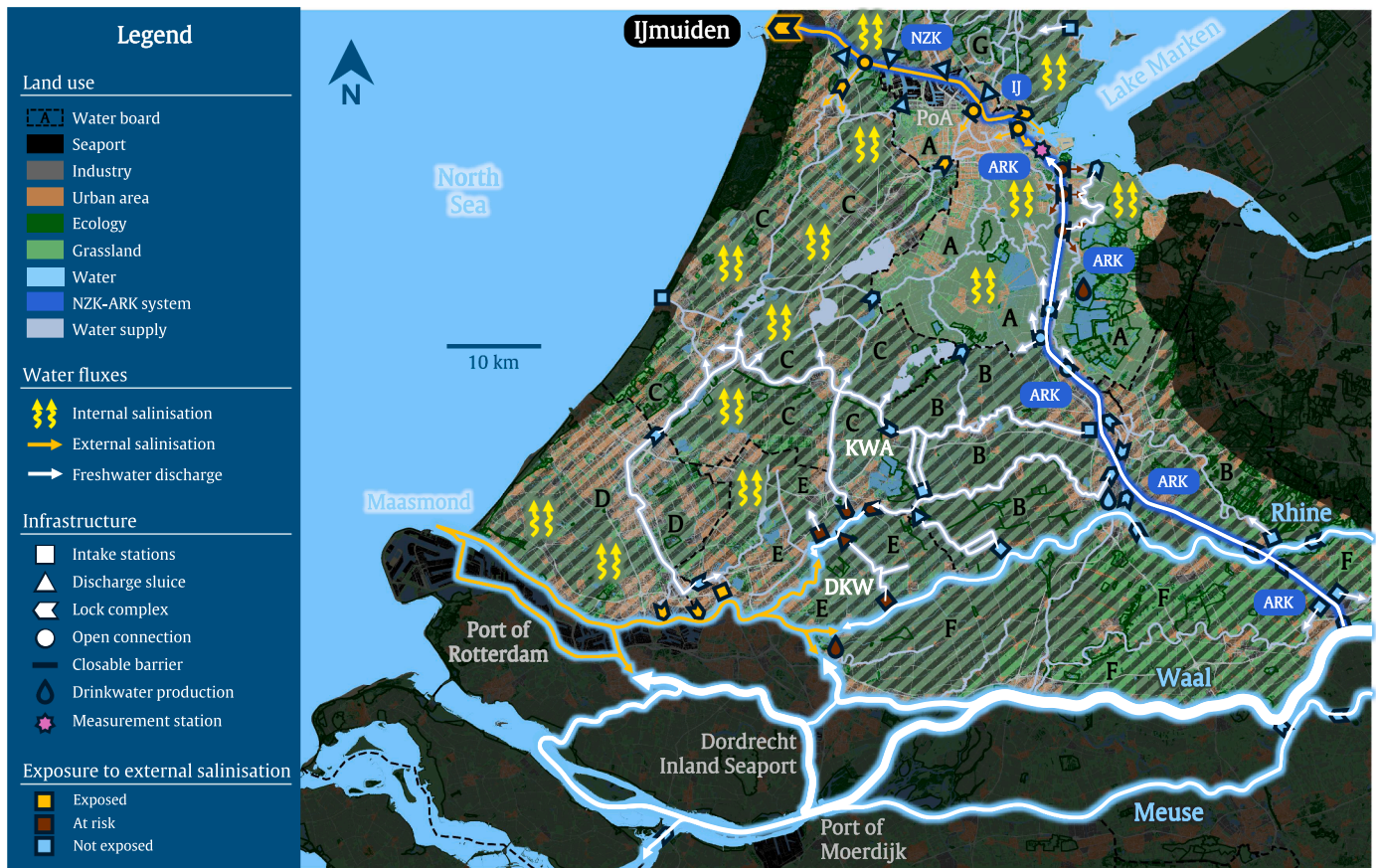
Fig. 1. Overview of the study area in the Rhine–Meuse Delta. Freshwater must be allocated to combat saltwater intrusion (orange arrows) through the Maasmond and the NSC–ARC system, driven by lock operations at IJmuiden (top of the figure), while also meeting the demands of users: drinking water, water safety, agriculture, and industry. The width of the freshwater discharges (white arrows) roughly represents the distribution of river discharges during droughts. The directly affected waterboard (light area) by the lock operations is A Waterschap Amstel, Gooi, Vecht; indirectly affected waterboards (shaded areas) are: B Hoogheemraadschap De Stichtse Rijnlanden, C Hoogheemraadschap van Rijnland, D Hoogheemraadschap van Delfland, E Hoogheemraadschap van Schieland and the Krimpenerwaard, F Waterschap Rivierenland, and G Hoogheemraadschap Hollands Noorderkwartier.
