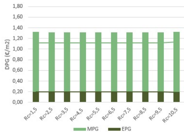
Figure 52: EPG and MPG of insulation value (EPG and MPG in column are stacked, and the lines represent the trend in EPG and MPG separately)
