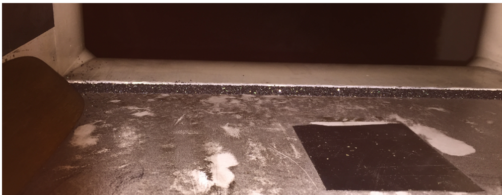
FIGURE A.2: Carborundum strip (width = 2 cm) at x = -975 mm just after the tunnel contraction to assure turbulent boundary layer.
