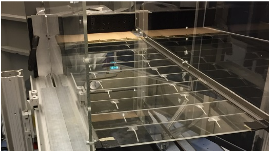
FIGURE A.4: Tufts on each individual sliding plate contained inside the planar diffuser.
