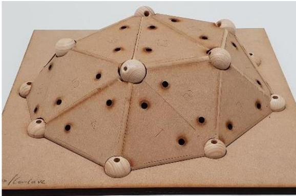
Figure 129 sphere at the nodes as a solution for transitioning between connection direction
