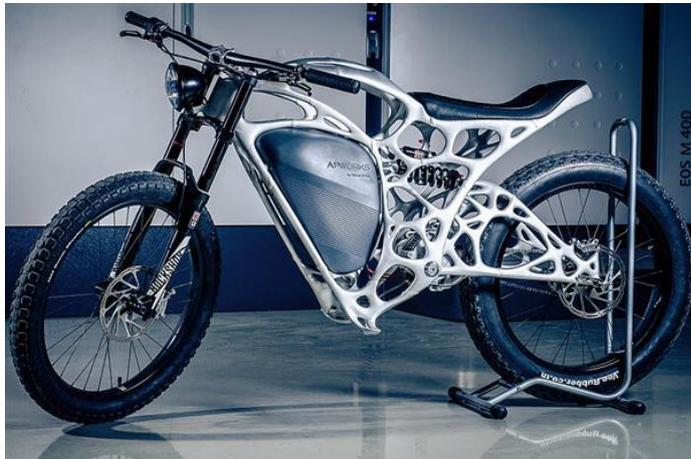
Figure 52 Light Rider: The 3D printed TO motorcycle (Grolms, 2016)
