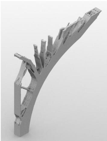
Extrusion of silhouette of 2nd optimised geometry
