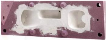
*Figure 149 Applied crystal cast coat for a smooth finish (Bhatia, 2019)*
