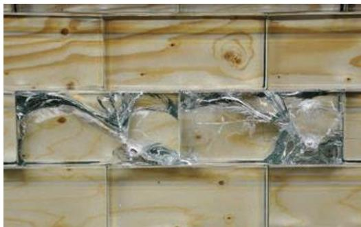
Figure 153 Vandalism test result (Oikonomopoulou, 2019)
