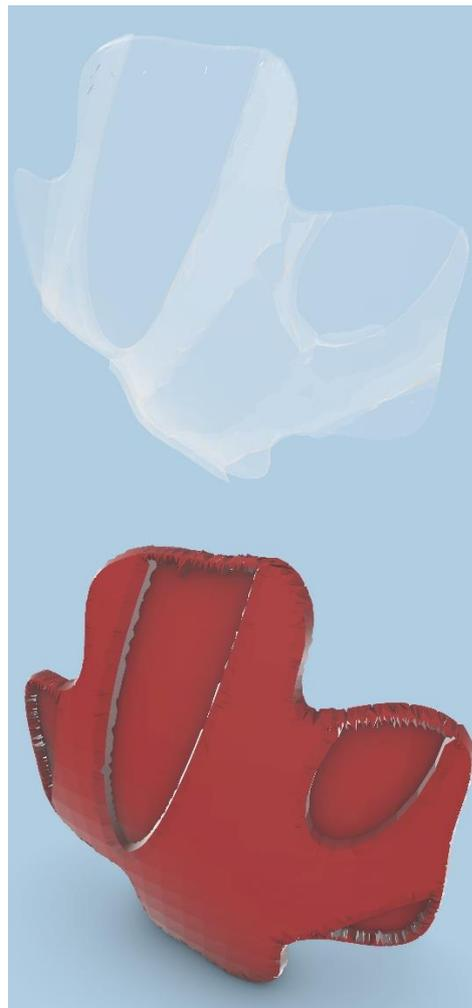
The relief on the exterior of the mould will be smoothed. This ensures manually added sand will slide easily filling all gaps.
