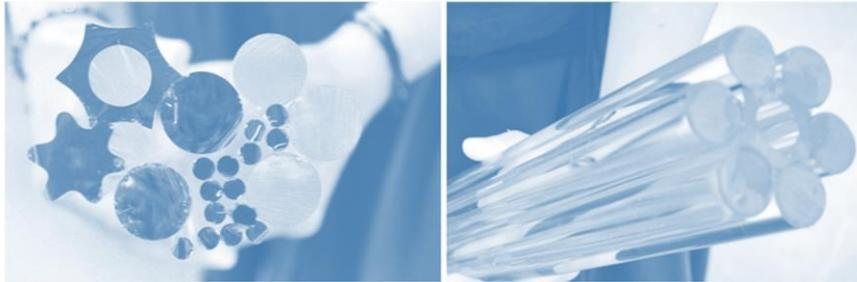
Figure 18 Right: Extruded glass bundled column with adhesive bond. Left: CONTURAX® and DURAN® extruded profiles by SCHOTT 2012 retrieved from Oikonomopoulou et al., 2017b
