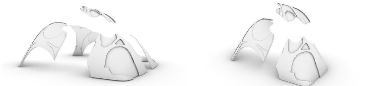
The division can be done based on a variety of reasonings. First, one might subdivide the shell into elements of max 40 kg so that they can be lifted by 2 people. Or, second, subdivided based on transportation dimensions limitation and production mould size limitations. With the second approach large pieces will be produced. More research has been conducted on brick-like glass structures than giant elements. Therefore, the second approach was adopted.
