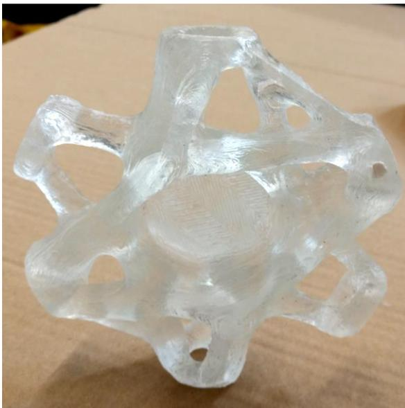
Figure 58 Casted TO node for light structure (Damen, 2019)
