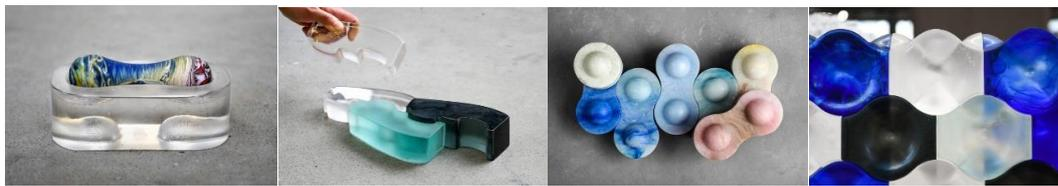
Figure 122 A variety of demountable dry-assembly structural cast glass interlocking systems as investigated by Oikonomopoulou et al. (2018a).
