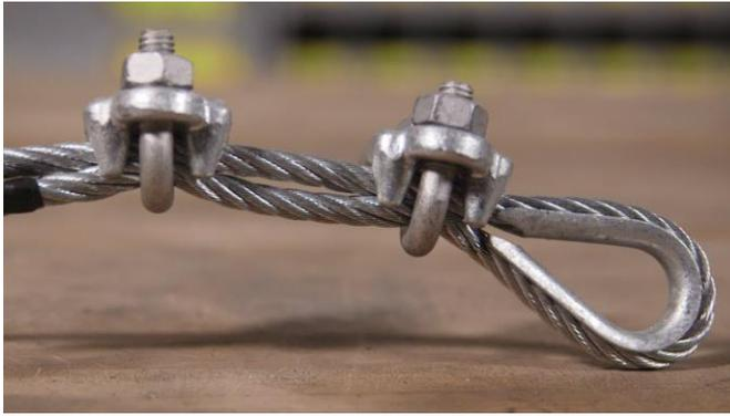
Figure 144 wire rope clipper. rope knotted into a loop (Kimball Midwest, 2018)
