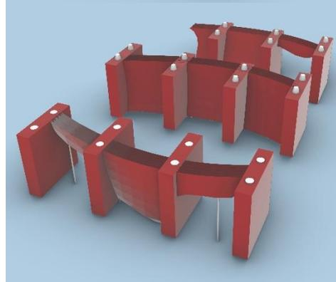
The sand mould will be additively manufactured using CHP binder system. Bhatia (2019) concluded that CHP was the most suitable binder for this project. This is because it loses its strength when exposed to high temperatures for a long time. It is also water solubility. These characteristics make it easy to detach the cast glass element from the mould. It makes it ideal for a one time use of mould. Image source VX4000 (VoxelJet, 2018b)
