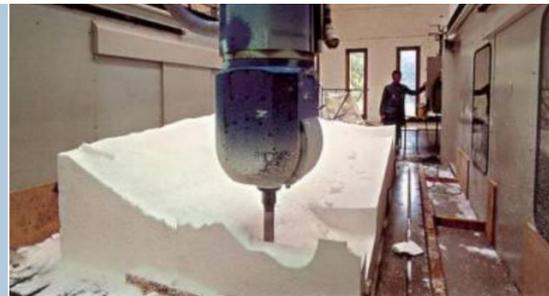
Figure 120 CNC milled formwork of Styrofoam to support shape negative shape of shell elements in wooden boxes transported in trucks
