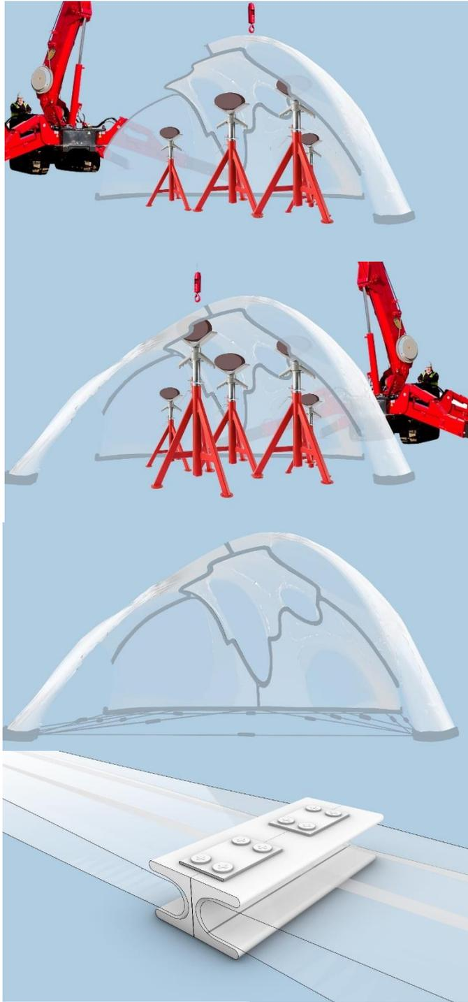
7. Connect the foundation cables and but do not fully tighten them.
