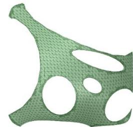
Figure 88 Simplified TO result with elliptic holes
