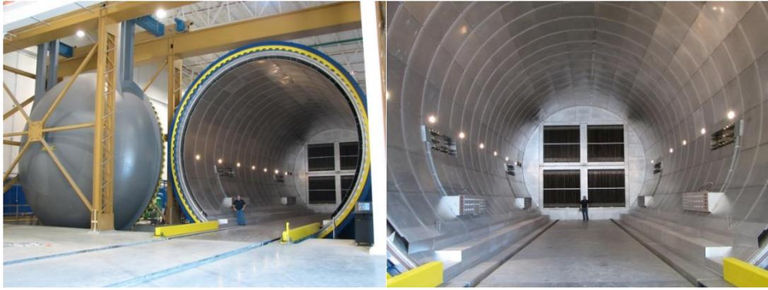
Figure 147 ASC Process Systems is the manufacturer of the World's Largest Autoclave System. Inside working diameter: 30ft. (9.26M). Inside working length: 76 ft. (23.5M)
