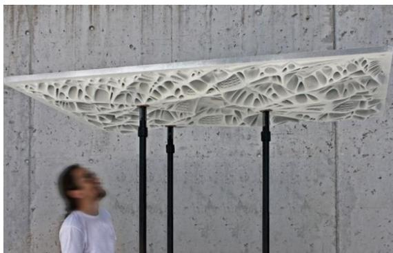
Figure 50 Prototype A ETH Zurich used the Millipede plugin for grasshopper for TO for this slab. Supported by 3 points. (Berhard et al., 2019)
