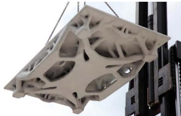
Figure 51 Prototype B ETH Zurich slab ABAQUS software was used for TO. It is designed to be supported at the four corners (Jipa et al., 2016)
