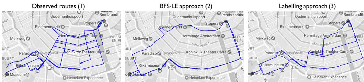
Figure 6.6: Routes generated for a given OD pair from Waterlooplein to Vondelpark, for (1) observed routes, (2) BFS-LE approach and (3) Labelling approach.
