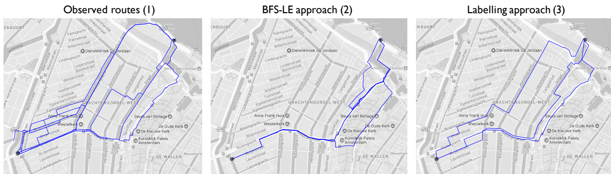
Figure 6.5: Routes generated for a given OD pair from the West of Amsterdam to the central train station, for (1) observed routes, (2) BFS-LE approach and (3) Labelling approach.
