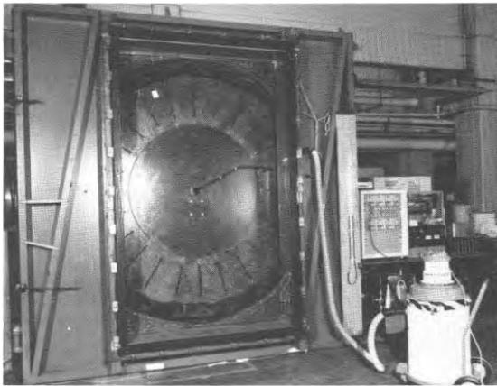
Figure 3.5: Front view of dynamic glass testing rig showing the 2.35m diameter piston behind the opening where the glass will be installed (Dalgliesh and Taylor, 1990).
