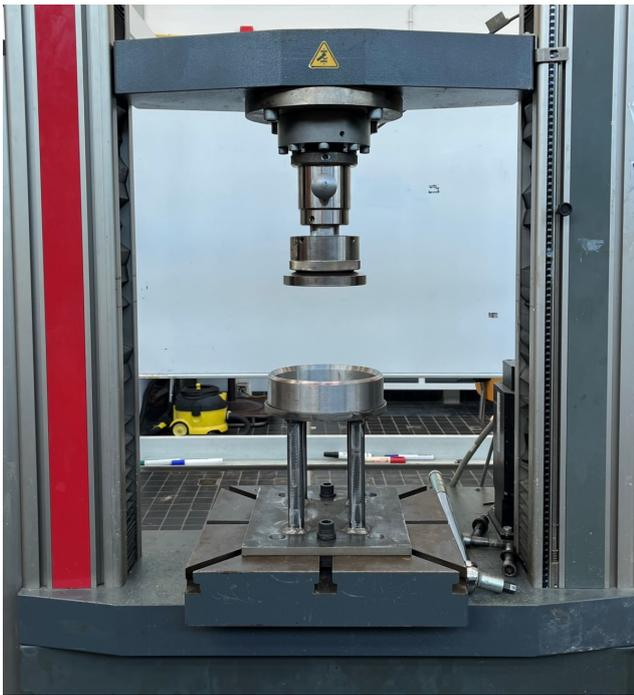
Figure 4.10: Materials testing machine Zwick Z100 at the Faculty of 3ME, TU Delft.
