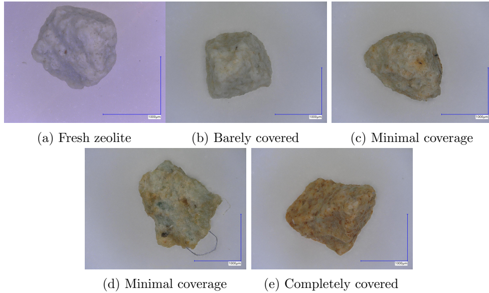
Figure 5.9: Microscopic pictures of zeolite with biofilm (except image a which is fresh zeolite) taken on 31.07.2023 at the end of the above-mentioned experiment. The nitrifying biofilm can be spotted by the brown tint on the zeolite surface which is otherwise greyish-white in color.
