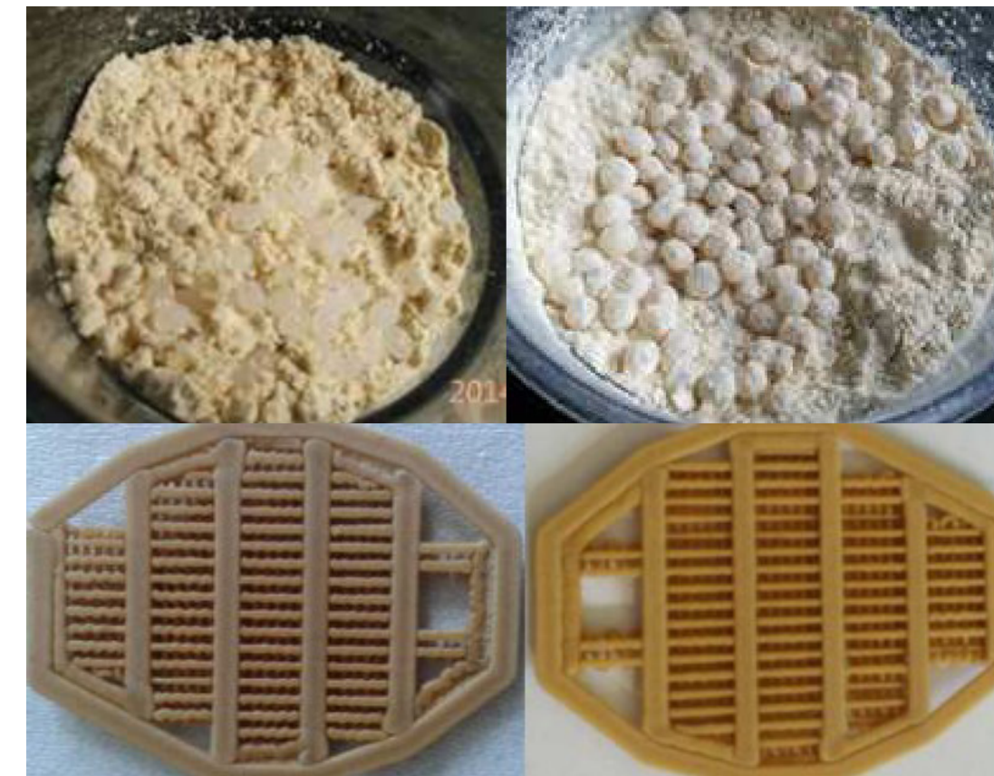
Premixing bamboo powder with PLA and comparison of different adding proportion.
