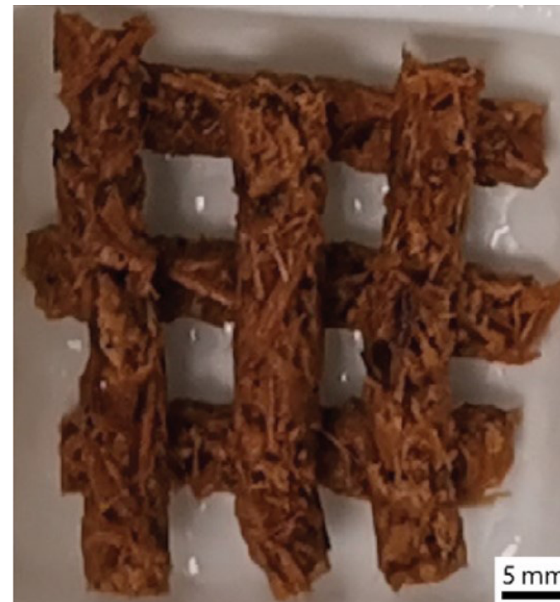
Extrusion of mycelium-enriched bamboo fibres-chitoan pastes.
