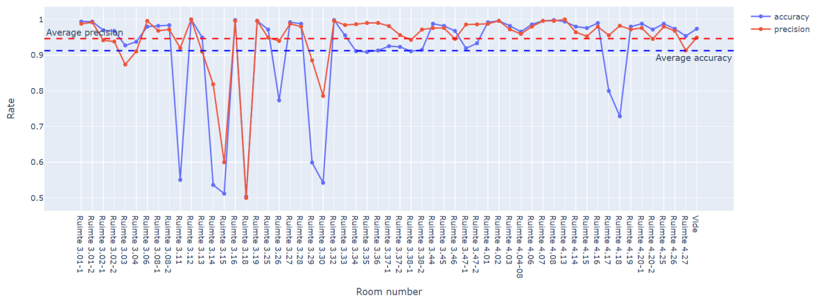
Figure 5-11: Accuracy and precision of detecting the mix of both anomaly, with the proposed classifier
