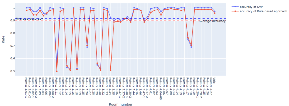
Figure 5-3: Accuracy of detecting the bias anomaly, with the proposed classifier and rule-based approach
