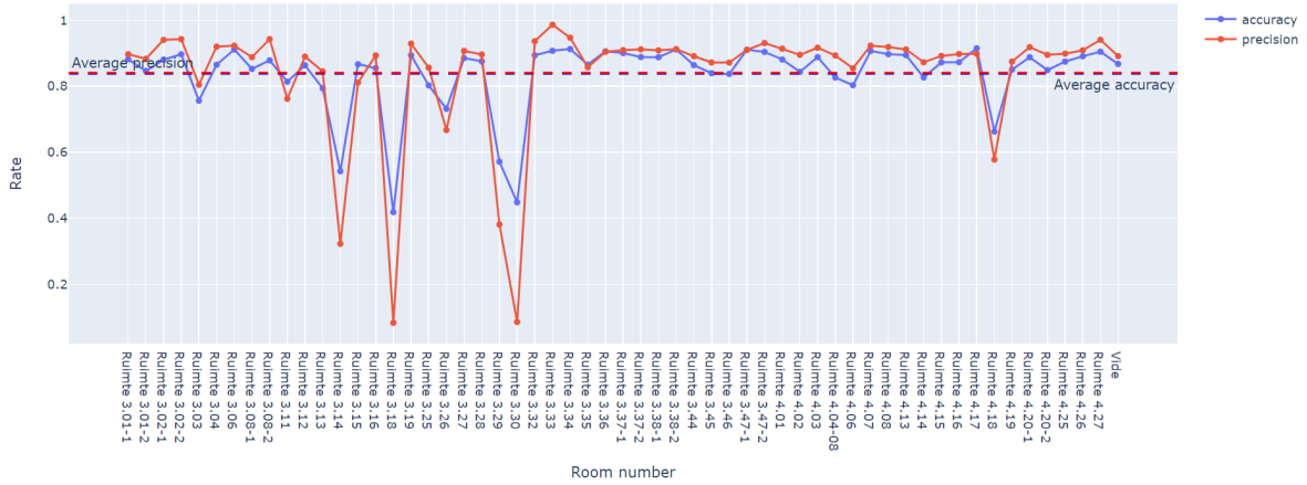
Figure 5-23: Average accuracy and precision of detector, based on the varying training room
