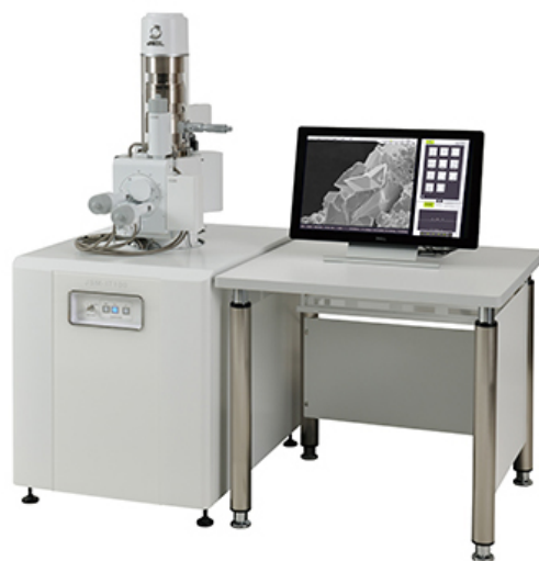
Figure 3.4: Jeol JSM-IT100 scanning electron microscope (SEM) used during analysis. This machine was also used for energy dispersive X-ray spectroscopy (EDS) results.
