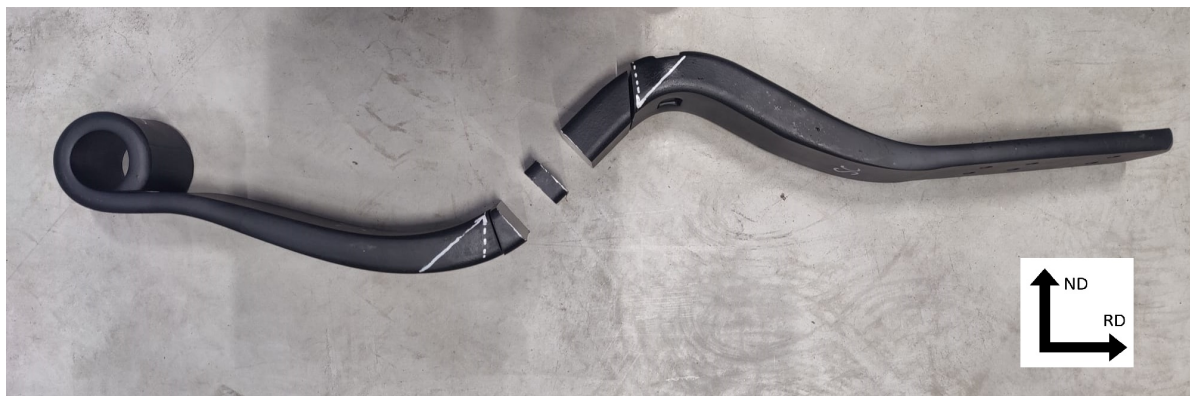
(a) Sample extraction form trailing arm.
