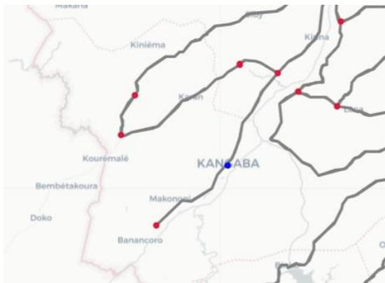
Figure 13. Example where a city (blue dot) lies on the road network but no node (red dot) is near.
