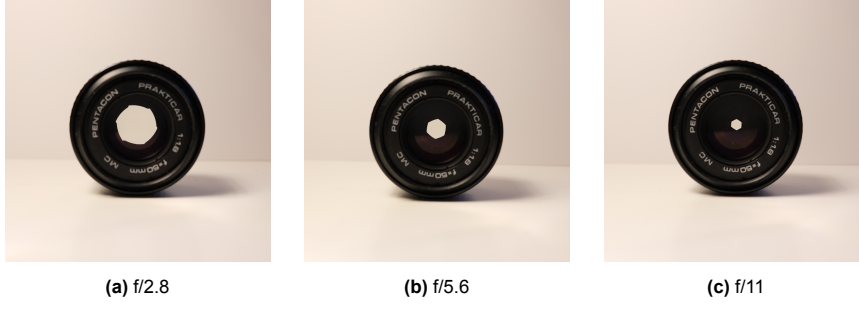
Figure 4.5: Aperture shape of the Pentacon Prakticar 50mm f/1.8 at different aperture settings.
