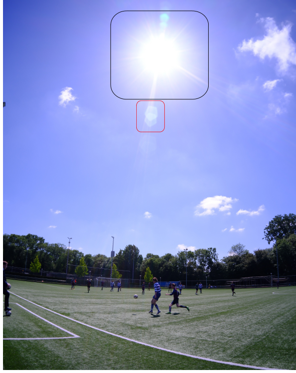
Figure 2.2: Real world flare artefacts example with the AstrHori 10mm f/8 II lens. The red square highlights ghost flares, and the black square highlights glare.
