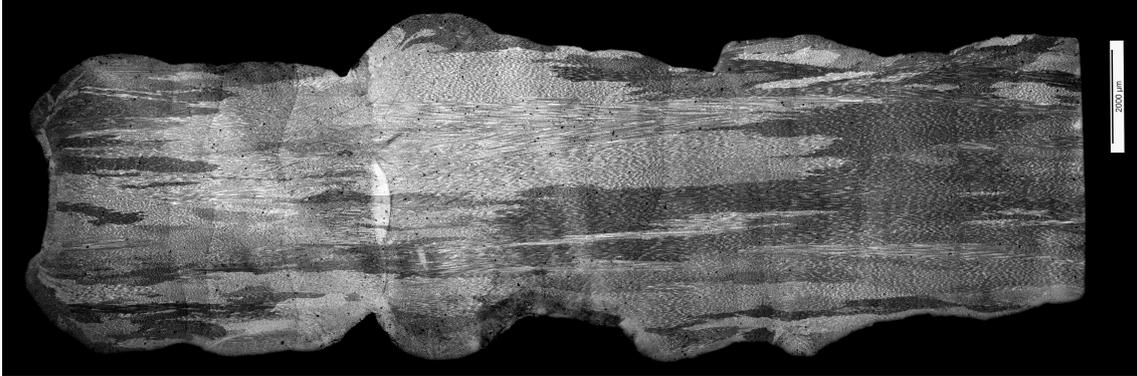
(a) Microstructure of specimen type 4-00
