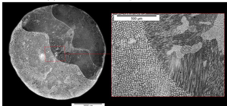
(c) Microstructure of specimen 2-60-A
