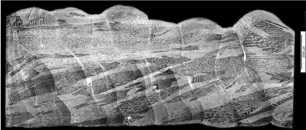
(c) Microstructure of specimen 2-60-A
