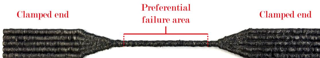
Figure 5.7: Fatigue test specimen
