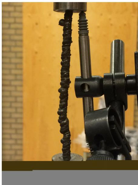
Figure 5.6: Hinged buckling test set-up
