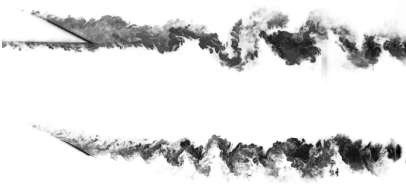
Figure 1.6: Smoke visualization of wake flow behind a beveled trailing edge. Images provided courtesy of S.C. Morris, University of Notre Dame.
