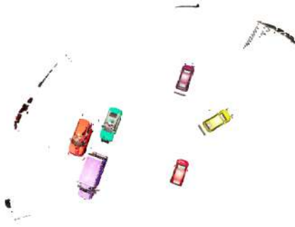
Fig. 7. The figure illustrates the need to account for points visible through vehicle windows. The left image shows the vehicles with many environmental artefacts around them, now considered part of the vehicles. Only associating points within the 3D bounding boxes of particular vehicles results in the right image, with most artefacts removed.
