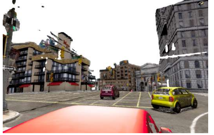
Fig. 13. The figure illustrates a triangle mesh representation of a traffic scene without simplifying the point clouds and triangle meshes. Not simplifying these representations makes the environment around the vehicles substantially less noisy compared to our mesh representations but increases computational expenses with the differentiable renderer.
