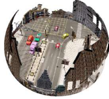
Fig. 6. The figure illustrates the usefulness of the spherical environment representation. The left image shows the result of not accounting for the distance of points from the ego vehicle, creating a large-scale point cloud representation. The right image shows the result of our spherical representation, where a sphere around the environment represents the environment beyond the representation radius. This spherical representation mitigates the size of the point cloud whilst keeping elements outside of the representation radius part of the traffic scene.
