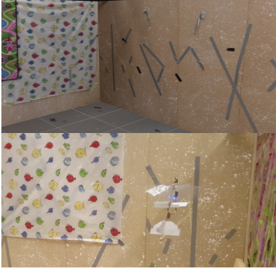
Fig. 2. Top: screenshot showing the simulated environment. Bottom: photo of the Delfly flying in the test room. The simulated room is an imitation of the real test room.
