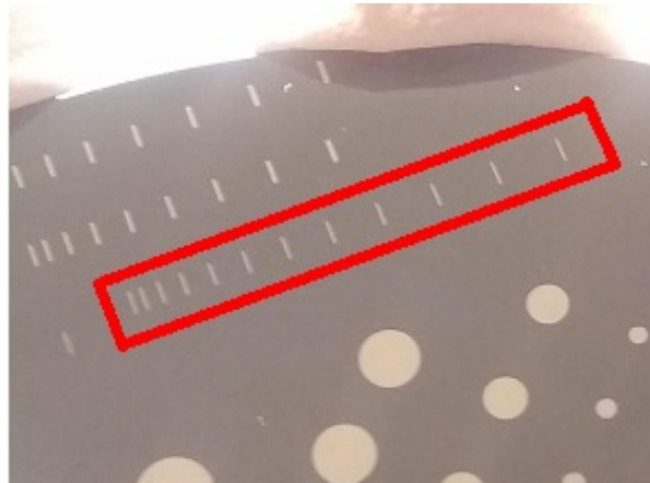
Figure 6.5: TLM pattern used to measure contact resistance of 6, 9, 12, 15 and 18 [min] tunnel oxides on n-type flat wafers. Highlighted in red are the 1 \mu\text{m} Al fingers used for the measurements.
