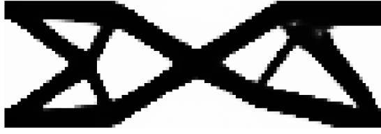
(a) Local optimum, found when using Ritz vectors ( n = 50 ) and PI penalization. The objective function is 6% higher than for the global optimum (Fig. 6.1d). Thus for this numerical example penalization was disabled.
