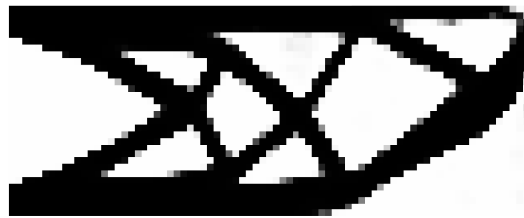
Figure 6.3: Structure optimized using modal superposition method with 100 basis vectors. The force is applied to the top-right corner, note that the optimization removes material around that area. The optimization was run for 500 iterations, but was still not converged. The resulting objective function is 3.15 times higher than the one associated with the optimal design. Total CPU-time is 1.3 times larger than the full optimization.
