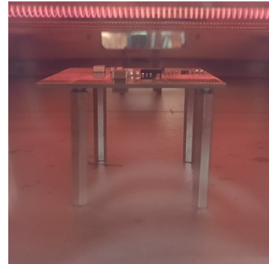
Figure 6.2: Evaluation board in the oven with metal stand-offs.
