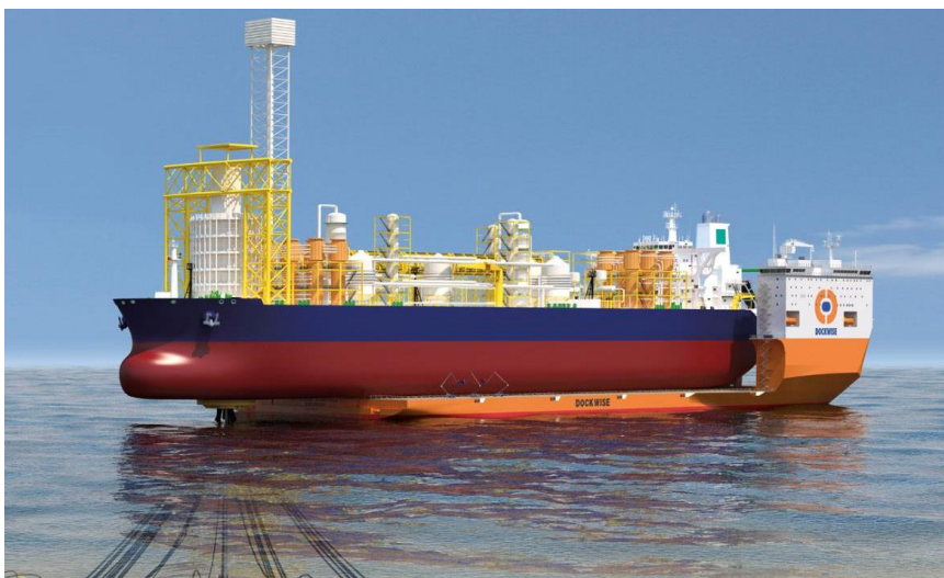
Figure 4: Offshore Dry-Docking of FPSO
