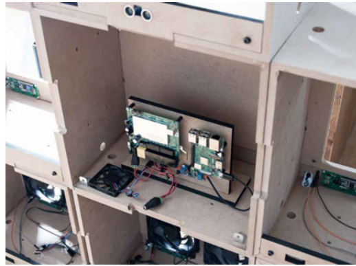
FIG. APP.D.18 Router and server built into the technical support module
