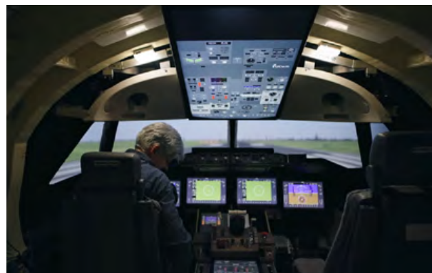
Figure 8: The full-motion research simulator SIMONA (Credits: Oculus Film)
