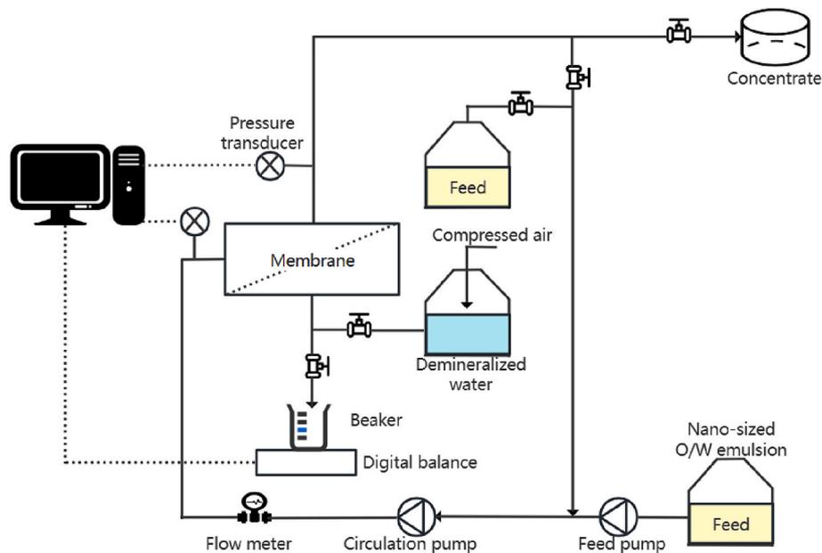
Fig. 1. Schematic diagram of constant flux filtration system.
