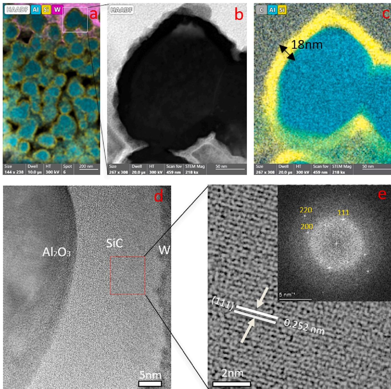
**Fig. 5.** (a) STEM EDX net intensity maps of the cross section of the H20 membrane. (b) STEM images and (c) EDX net intensity maps of a SiC coated alumina particle near the top. (d) and (e) High-resolution TEM images of the H20 membrane with SAED patterns (upper right).
