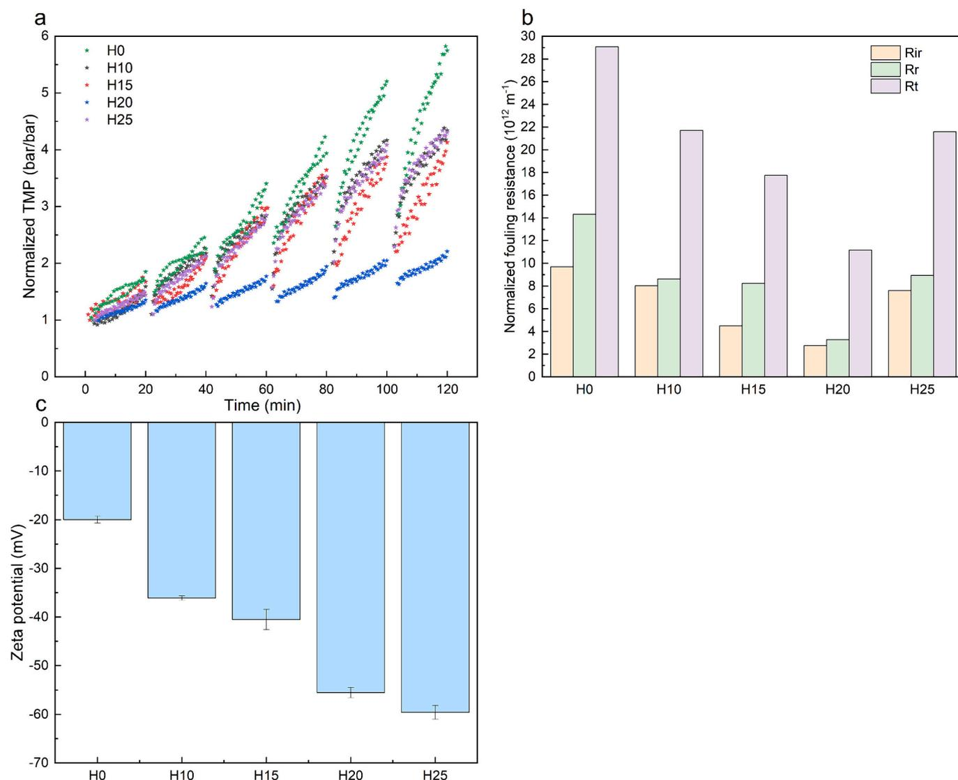
**Fig. 8.** The normalized (a) TMP and (b) fouling resistance of the H0, the H10, the H15, the H20, the H25 membrane for the filtration of microemulsion (500 mg/L soybean oil with 50 mg/L Span 80 and 50 mg/L Tween 80); (c) is the zeta potential of the H0 the H10, the H15 the H20, the H25 membranes in the surfactant solution with 50 mg/L Span 80 and 50 mg/L Tween 80.
