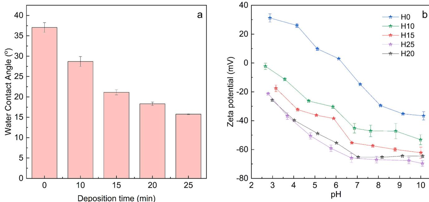
Fig. 6. Initial water contact angle (a) and zeta potential (b) of  $\text{Al}_2\text{O}_3$  membrane (H0) and SiC-coated  $\text{Al}_2\text{O}_3$  membranes (H10, H15, H20, H25) with increasing deposition times.
