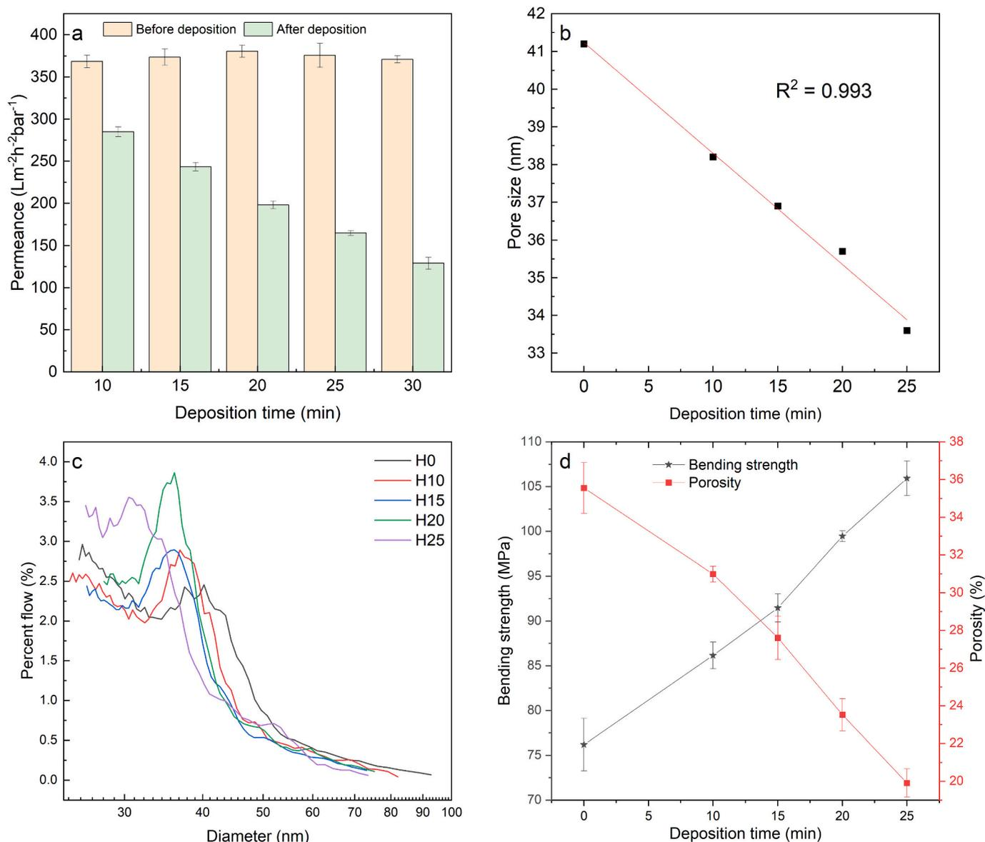
**Fig. 7.** (a) Permeance, (b) pore size, (c) pore size distribution, and (d) bending strength and porosity of the Al<sub>2</sub>O<sub>3</sub> membrane (H0), and the SiC-coated Al<sub>2</sub>O<sub>3</sub> membranes with increasing deposition times: H10, H15, H20, H25.
