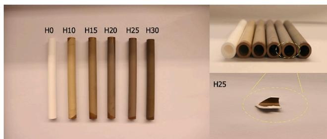
**Fig. 3.** Photographs of the Al<sub>2</sub>O<sub>3</sub> (H0) membrane and SiC-coated Al<sub>2</sub>O<sub>3</sub> (H10, H15, H20, H25) membranes.
