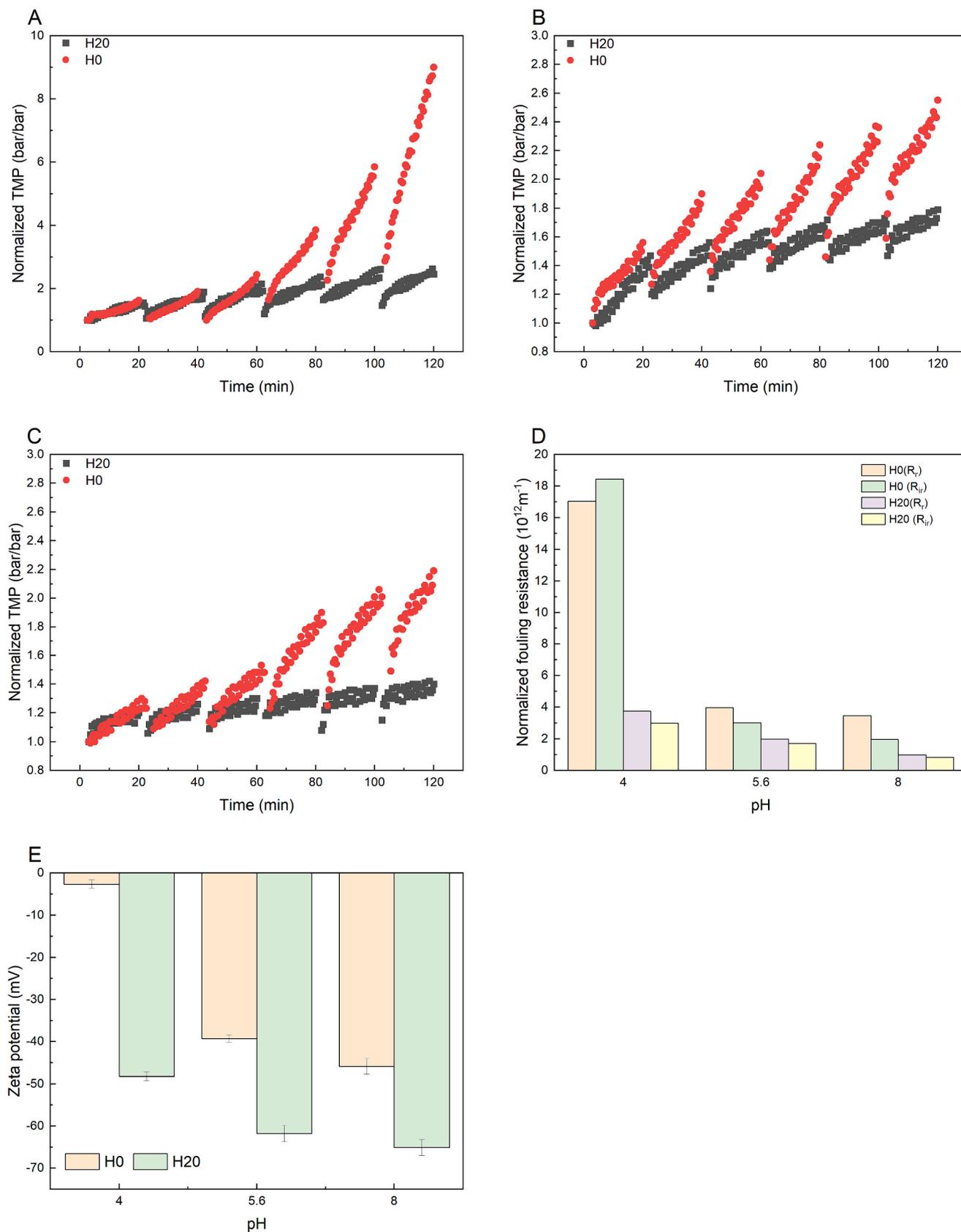
**Fig. 9.** Normalized TMP of the H0 and the H20 membrane or the filtration of microemulsion stabilized with 50 mg/L Span 80 and 50 mg/L SDS at the pH of (a) 4, (b) 5.6, and (c) 8; (d) is the normalized fouling resistance of the H0 and the H20 membrane at the pH of 4, 5.6 and 8; (e) is the zeta potential of the H0 and the H20 membrane at the pH of 4, 5.6 and 8.
