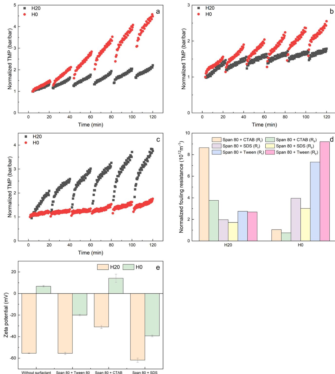
**Fig. 10.** Fouling comparison of the H0 and the H20 membrane during the filtration of microemulsions stabilized with various types of surfactant: 50 mg/L Span 80 and 50 mg/L (a) Tween 80, (b) SDS, (c) CTAB. (d) is the normalized fouling resistance of the H0 and H20 membranes at various surfactant types. (e) is the zeta potential of the H0 and the H20 membrane in different surfactant solutions.
