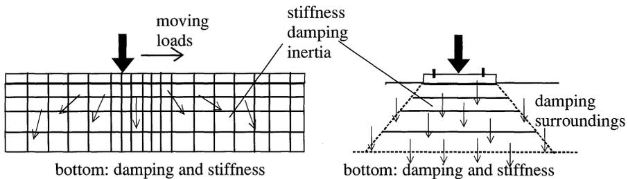
Fig. 3. Energy dissipation.
