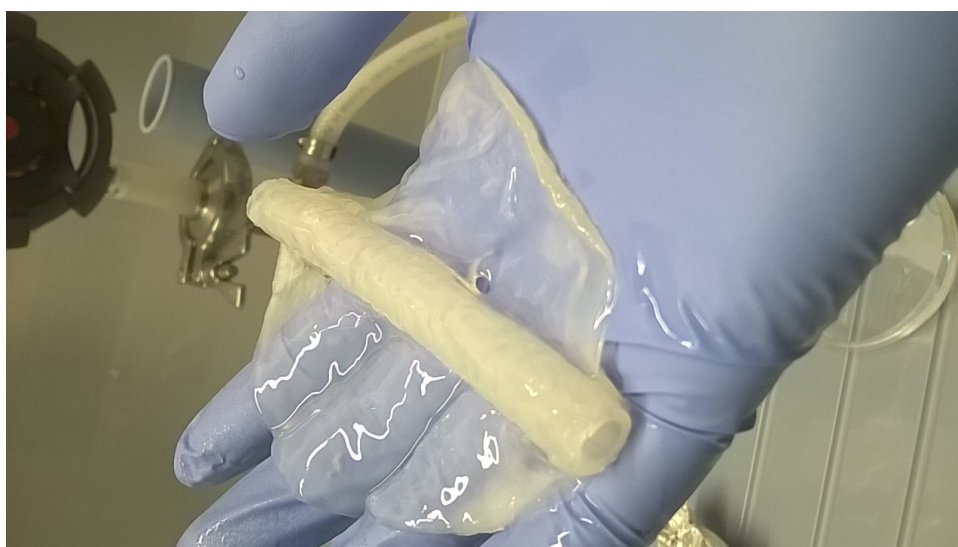
Fig. 5.1: The BC tube around the silicon tube after 6 days of culturing submersed in medium in a Petri dish. The surface patch has merged with the tube growing around the silicon
