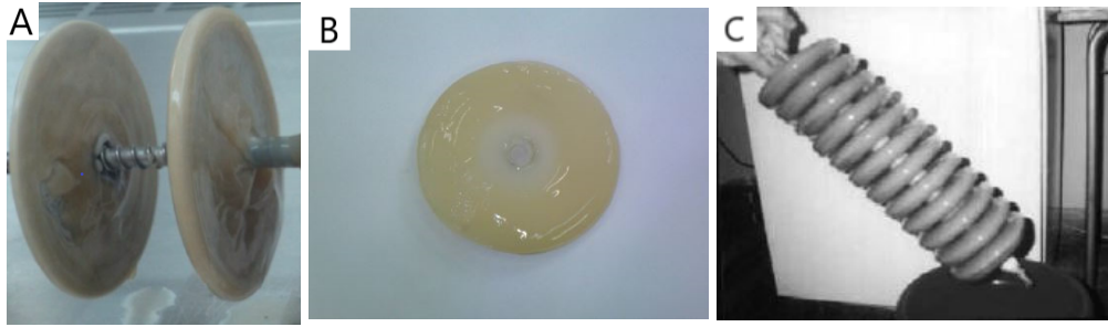
Fig. 4.2: Results on industrial rotation devices of (A) Lin et al. [38] on stainless steel for five days, (B) Kim et al. [34] on polypropylene for four days and (C) krystynowicz et al. [37] on polyethylene for seven days
