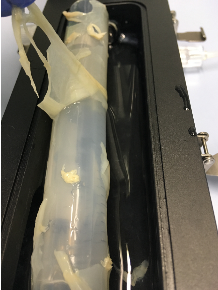
Fig. 4.2: Material structure of Rotary Test 4; a silicon tube
