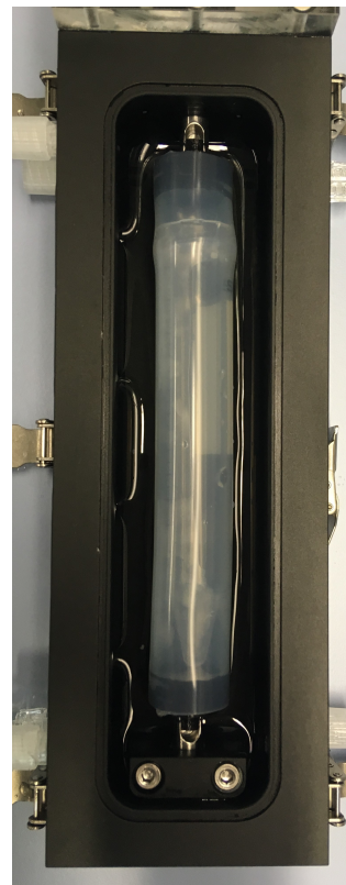
(b) Test 4 with a silicon tube. Two adapters connect the tube to the rotary device
