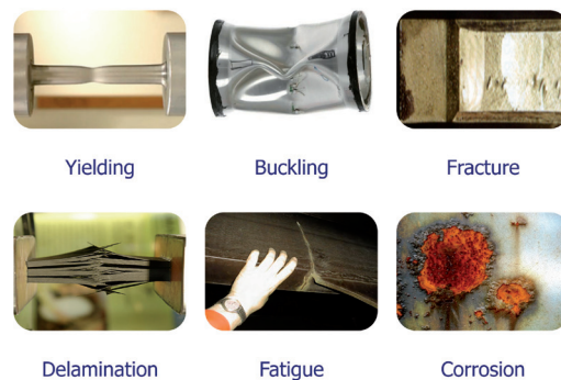
Figure 13. Basic structural failure modes. [28, 29, 30, 31, 32, 33]
