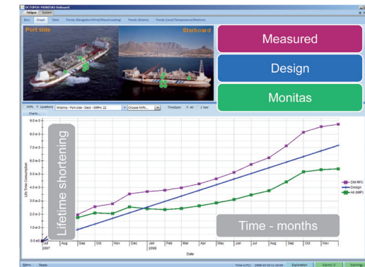
Figure 27. Lifetime consumption predicted by the Monitas system (video). [48]
