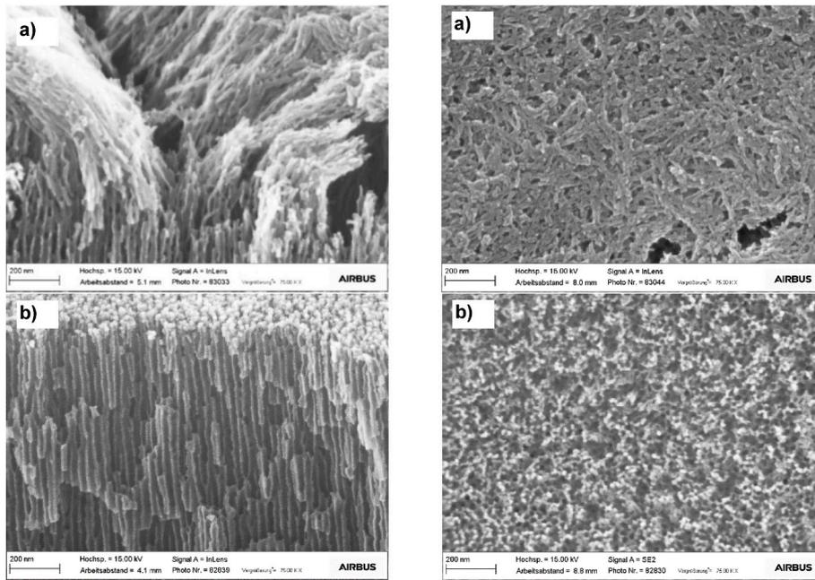
**Fig. 8.** FE-SEM images (cross-section) at the surface of the anodic oxide: a) Collapsed anodic oxide layer (SAA 14 V 55 °C) and b) Anodic oxide layer (T + SA 14 V 55 °C). Pre-treatment with acidic pickling in Bonderite C-IC SmutGo NC AERO.
