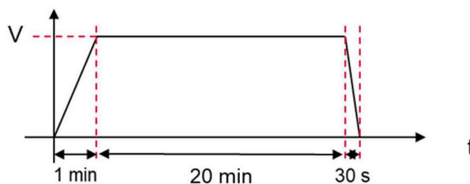
Fig. 1. Schematic view of the applied potential profile.
