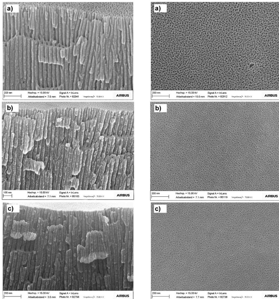
**Fig. 9.** FE-SEM images (cross sections) of anodic layers formed at 37 °C and 20 V in a) SAA b) TSA and c) T<sup>+</sup>SA (pre-treatment with acidic pickling in Bonderite C-IC SmutGo NC AERO).
