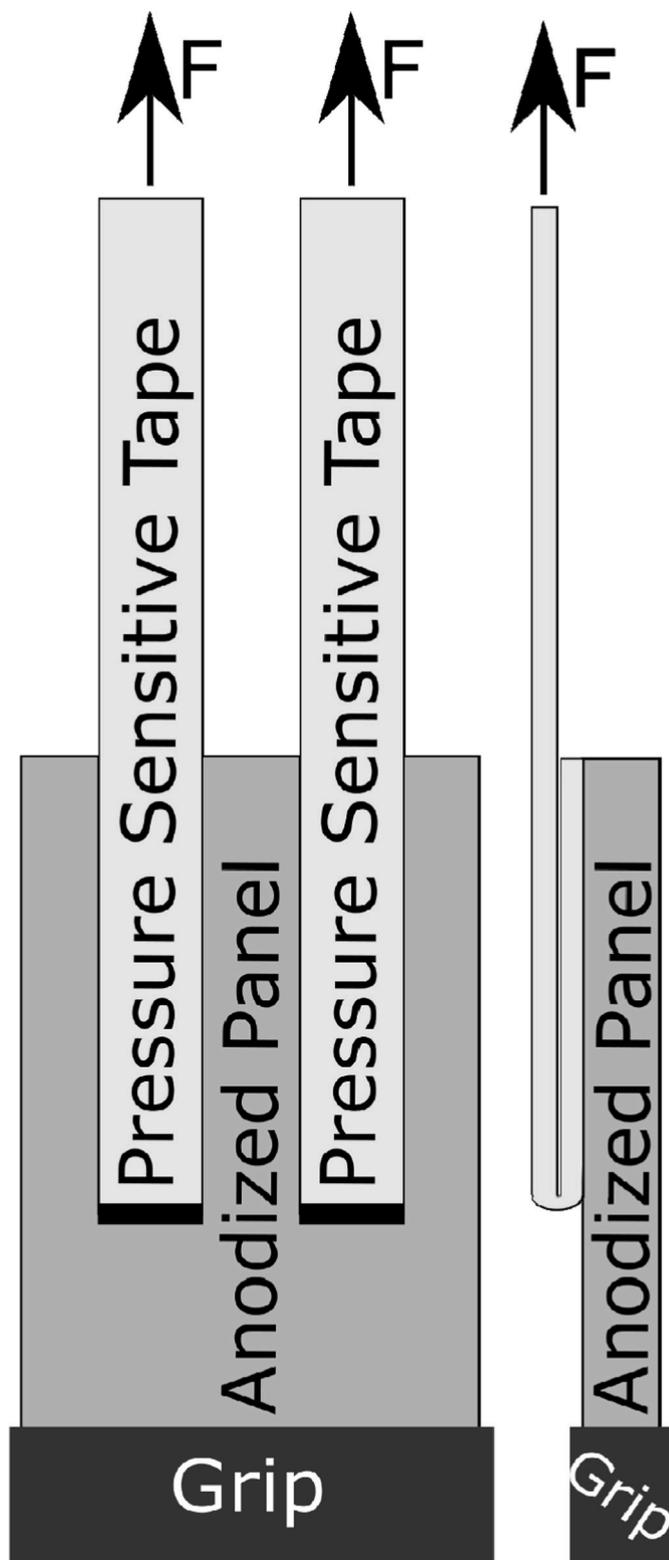
**Fig. 2.** Schematic representation of the adhesion test setup.
